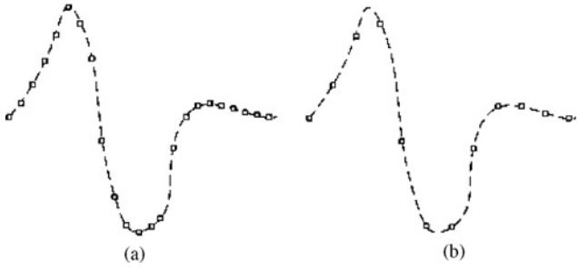
Fig. 4. Illustration of edge profile blurring by decimation. (a) Sampling of the edge profile. (b) Blurring of the decimated edge profile.
