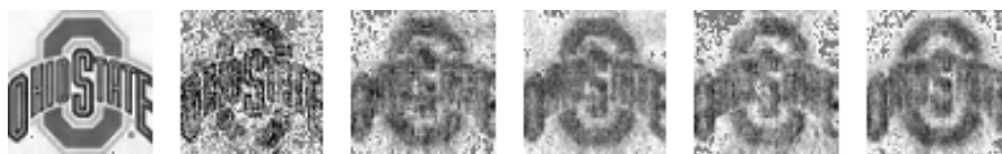
(b) Logo Two: 21.49dB (No Attack); 8.167dB (D=13.02dB); 8.13dB (D=16.88dB); 9.129dB (D=18.38dB); 7.569dB ( QF = 20 ); 8.9dB ( CR \approx 34 ).
