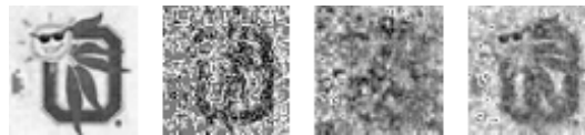
(c) Logo Three (Host Peppers): 19.97dB (No Attack); 7.541dB (AWGN D=12.98 dB); 7.8295dB (JPEG QF = 50 ); 10.34dB (JPEG2000 CR \approx 17 ).
