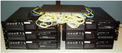
Fig. 9. Hardware testbed with 6 servers and 10 virtual switches configured with a production Pica8 48-port OpenFlow switch.
