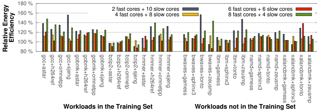
Fig. 2. Relative energy efficiency of our energy-efficient algorithm and the default Xen Credit Scheduler in 4 sets of core frequency settings.
