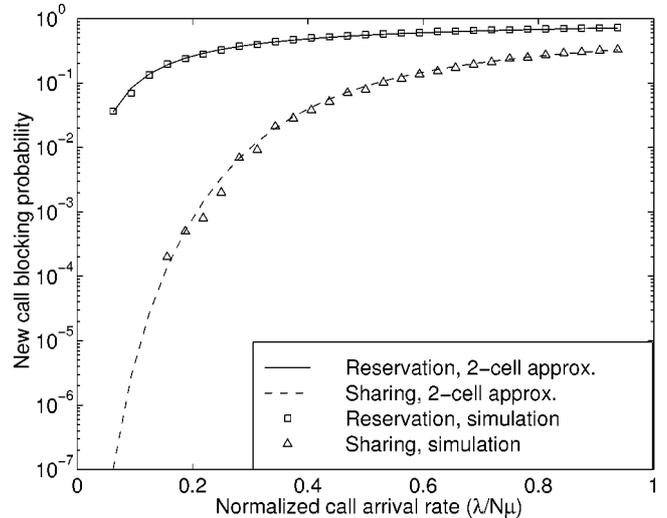
Figure 13. Comparison of new call blocking probabilities for the channel sharing handoff scheme and the channel reservation scheme (reuse factor  $r = 3$ ).
