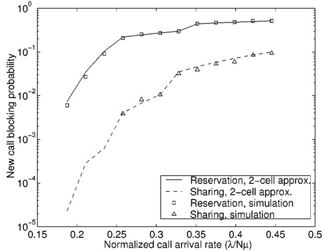
Figure 14. Comparison of new call blocking probabilities for the hybrid channel sharing handoff scheme and the channel reservation scheme (reuse factor  $r = 2$ ). The handoff dropping probability threshold is set at  $10^{-6}$ .
