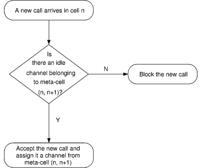
Figure 5. Flow chart for processing a new call.
