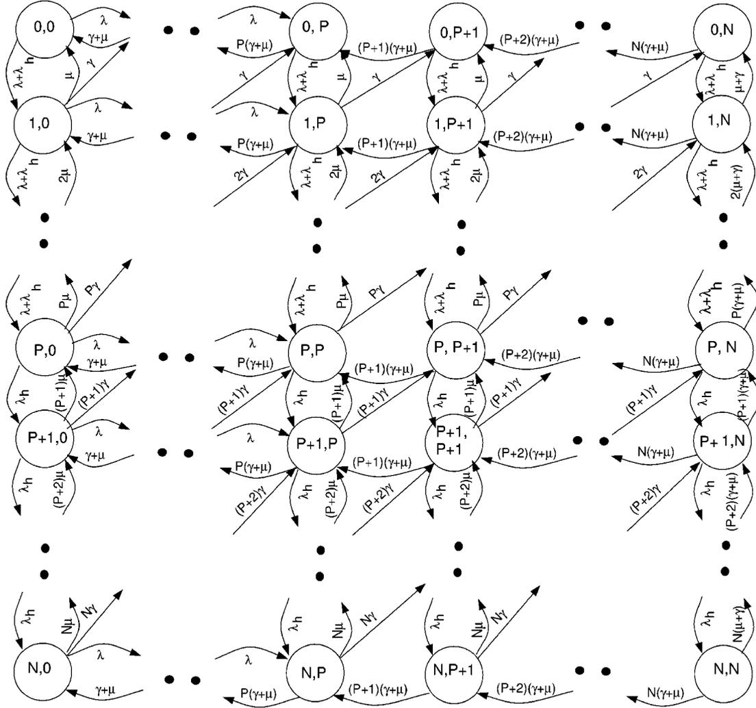
Figure 10. Continuous-time Markov chain of the two-cell approximation for fixed channel allocation with  $N - P$  guard channels.
