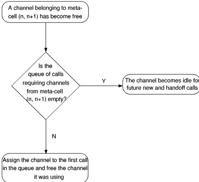
Figure 7. Flow chart for processing a freed channel.
