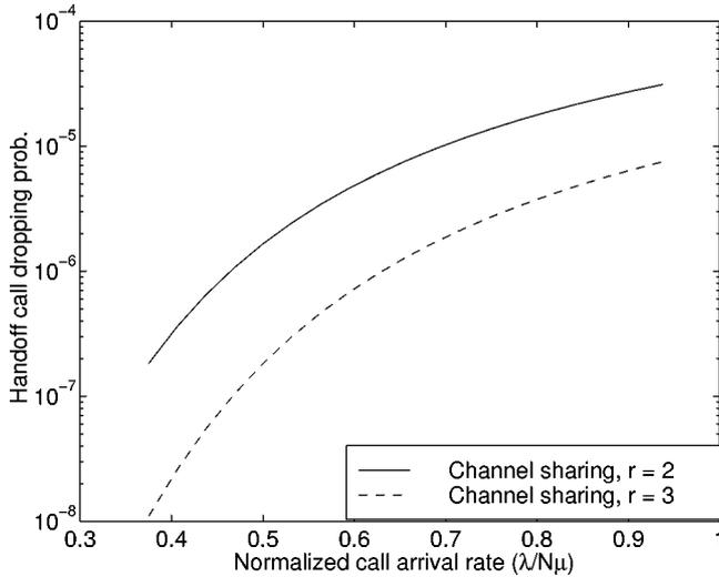
Figure 11. Comparison of two-cell approximations of handoff dropping probabilities for the channel sharing handoff scheme for reuse factors  $r = 2$  and 3.
