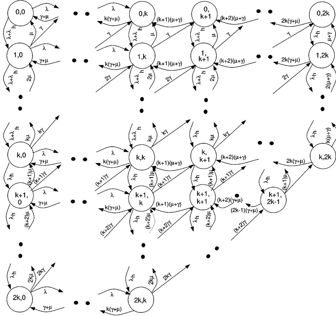
Figure 9. Continuous-time Markov chain of the two-cell approximation for channel sharing handoff scheme.
