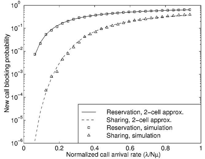
Figure 12. Comparison of new call blocking probabilities for the channel sharing handoff scheme and the channel reservation scheme (reuse factor  $r = 2$ ).
