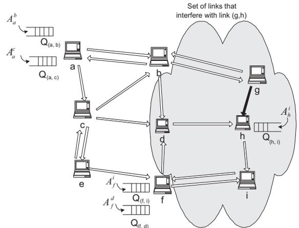
Fig. 1. Figure showing a wireless network with single-hop traffic. All packets  $A_s^d$ , transmitted on link  $(s,d)$  are exogenous and are queued ( $Q_{s,d}$  denotes the queue length). All the links that interfere with link  $(g,h)$  are shown.
