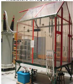
Insulators in fog chamber
