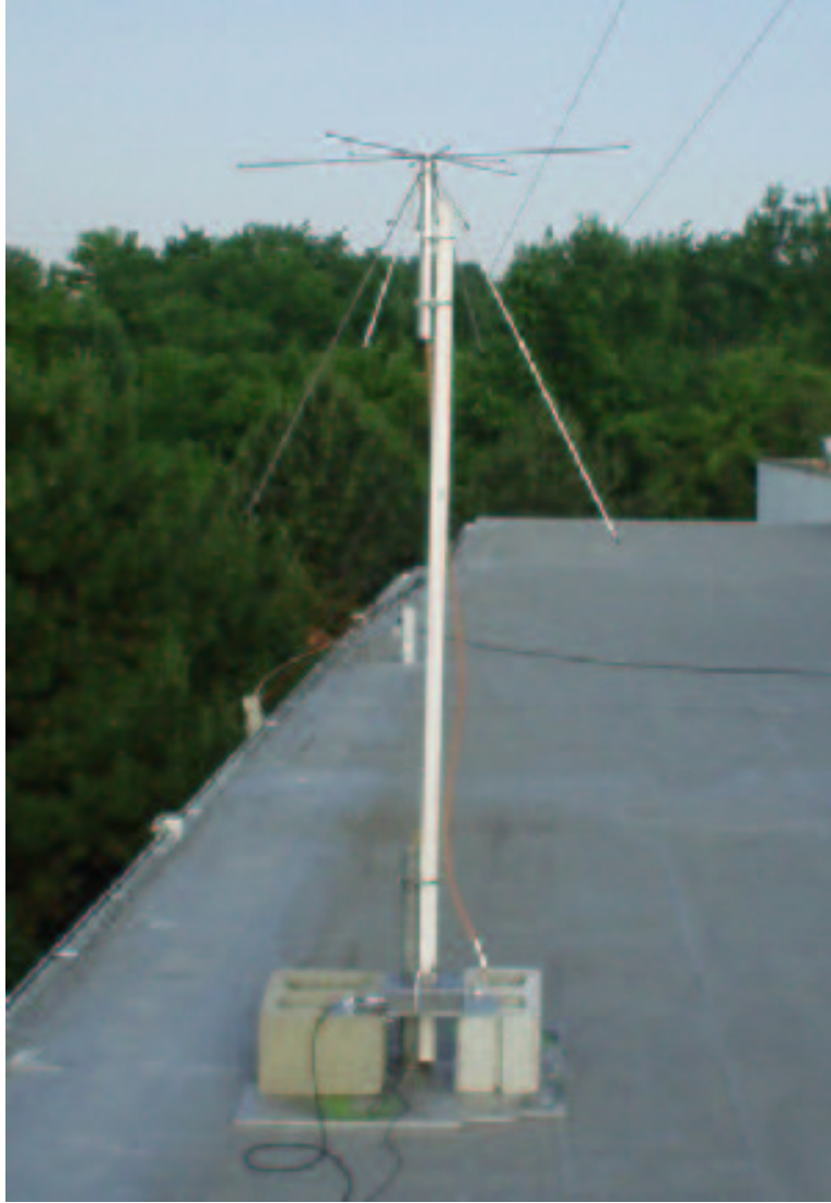
Figure 2: Antenna and front end box, as mounted on the roof of ESL. The antenna is about 10 m above ground level.
