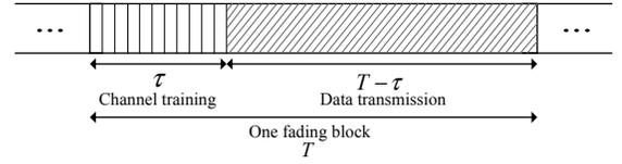
Fig. 3. A typical estimation - data transmission structure.
