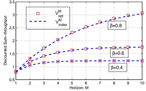
Fig. 7. Performance of the index policy in comparison with that of the optimal policy. System parameters used:  $N=5, \{p_1=0.2, r_1=0.75\}, \{p_2=0.6, r_2=0.25\}, \{p_3=0.8, r_3=0.3\}, \{p_4=0.4, r_4=0.7\}, \{p_5=0.65, r_5=0.55\}$ ; Fading block length:  $T=20$ .
