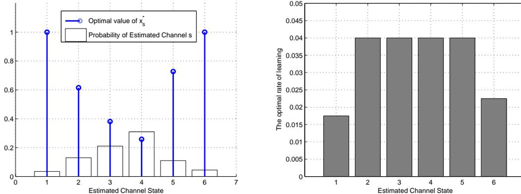
Fig. 3. Illustration of the design of optimal  $x_s^*$  when  $N = 2$ ,  $\gamma = 0.2$  and  $S = \{1, \dots, 6\}$
