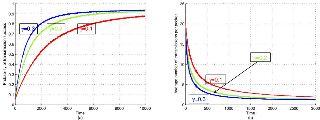
Fig. 4. Illustration of the time evolution of the (a) Probability of successful packet transmission (b) Average number of retransmissions per packet for various values of  $\gamma$ .
