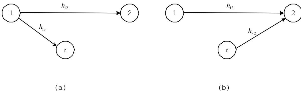
Fig. 3. The cooperation scheme in the small network: a) both the relay and node 2 keep receiving, lasting  $\mu T$  b) both node 1 and the relay transmit, lasting  $(1 - \mu)T$ .
