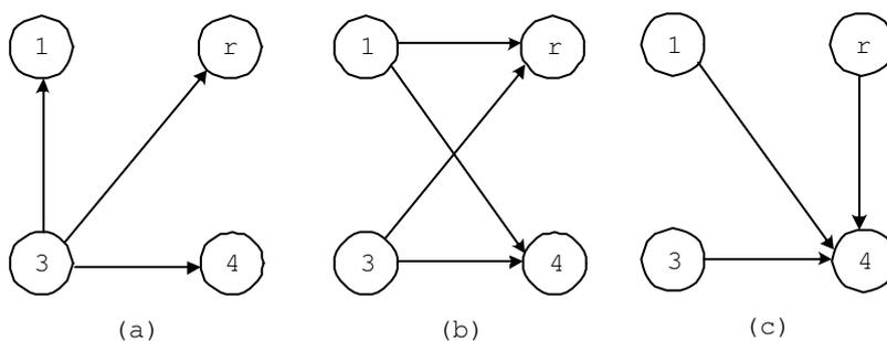
Fig. 4. The operation sequence when node 1 helps node 3 and  $h_{31} > h_{3r}$ , (a) node 1 and the relay keep listening, lasting  $\mu'_{3,1}T$  (b) node 1 helps transmitting, lasting  $\mu'_{3,2}T$  part of the time (c) both node 1 and the relay help, lasting  $(1 - \mu'_{3,1} - \mu'_{3,2})T$ .
