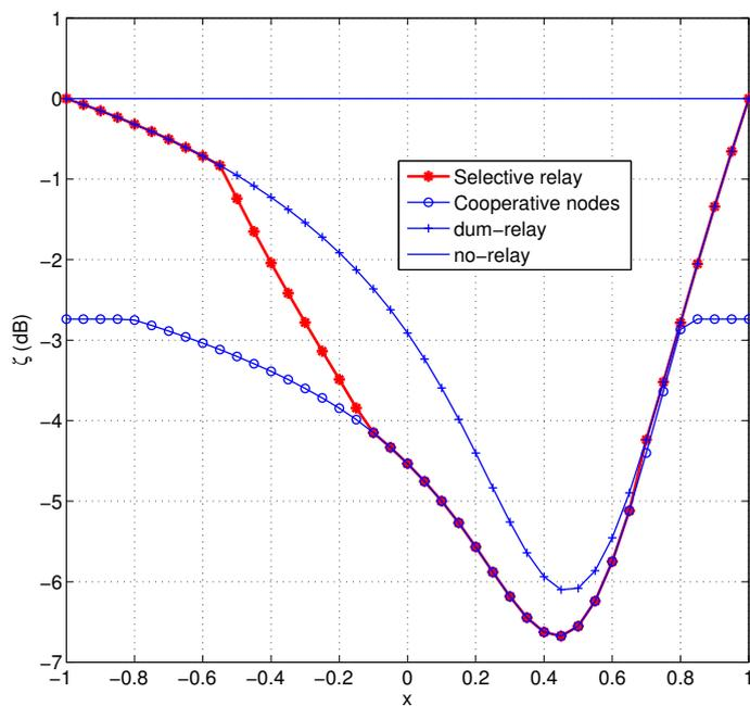
Fig. 7. Comparison between relay strategies (dumb relaying refers to the case where the relay always helps).
