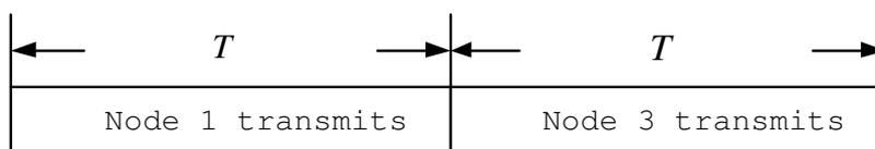
Fig. 2. The TDMA data frame.
