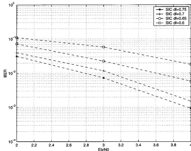
Fig. 5. Performance of the SIC receiver at different channel spacings with the four-state code.
