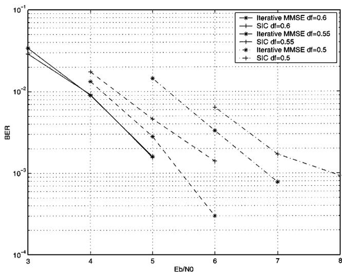
Fig. 3. Performance of the iterative mmse and SIC receiver at different channel spacings with the four-state code.
