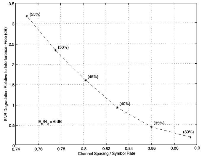
Fig. 2. Performance of the proposed subtractive interference canceler, when interference cancellation is done prior to FEC decoding, with varying levels of channel spacing.
