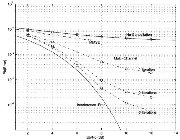
Fig. 1. Performance of the proposed methods at channel spacing of  $0.86T_s^{-1}$  when interference cancellation is done prior to FEC decoding. (Solid line: analysis; "o": simulation).
