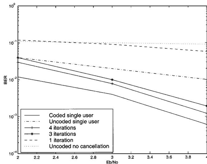
Fig. 4. Performance of the SIC receiver at channel spacing of  $0.75T_s^{-1}$  with the four-state code.
