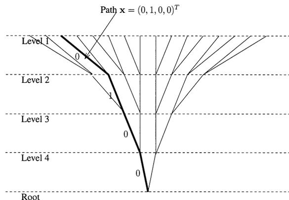
Fig. 1. Tree representation of the paths searched by the sphere decoder in the case  $m = 4$  and  $Q = 2$ . A particular path is evidenced as an example.
