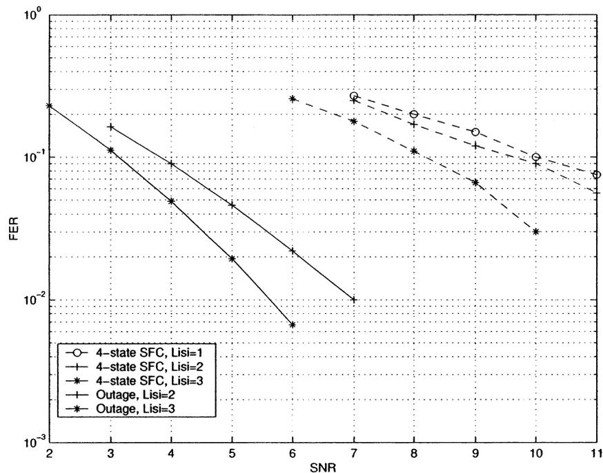
Fig. 4. Performance of four-state BPSK SFC with  $L_t = 2$ , and  $L_r = 1$ .
