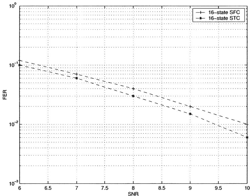
Fig. 8. Performance of BPSK STC and SFC with  $L_t = 3$ ,  $L_r = 1$ , and  $L_{ISI} = 2$ .
