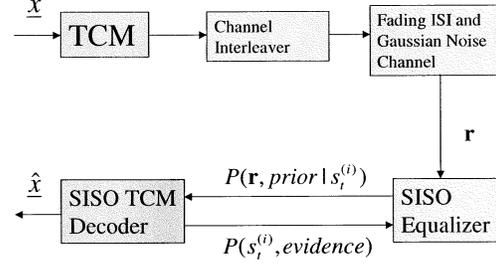
Fig. 2. Block diagram of the iterative receiver for the serially concatenated code.
