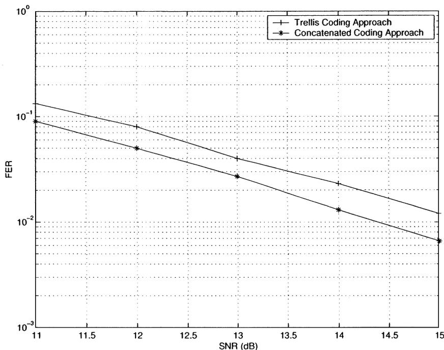
Fig. 13. Performance comparison of the serially concatenated coding approach and the trellis coding approach (QPSK).
