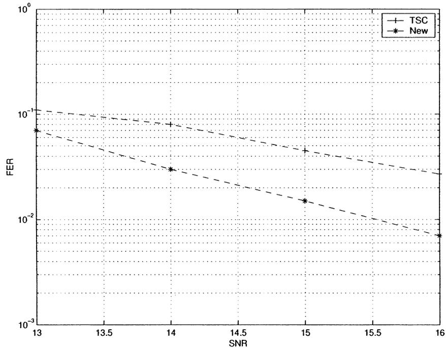
Fig. 12. Performance of two 16-state QPSK SFCs for  $L_t = 2$ ,  $L_r = 1$ , and  $L_{\text{ISI}} = 3$ .
