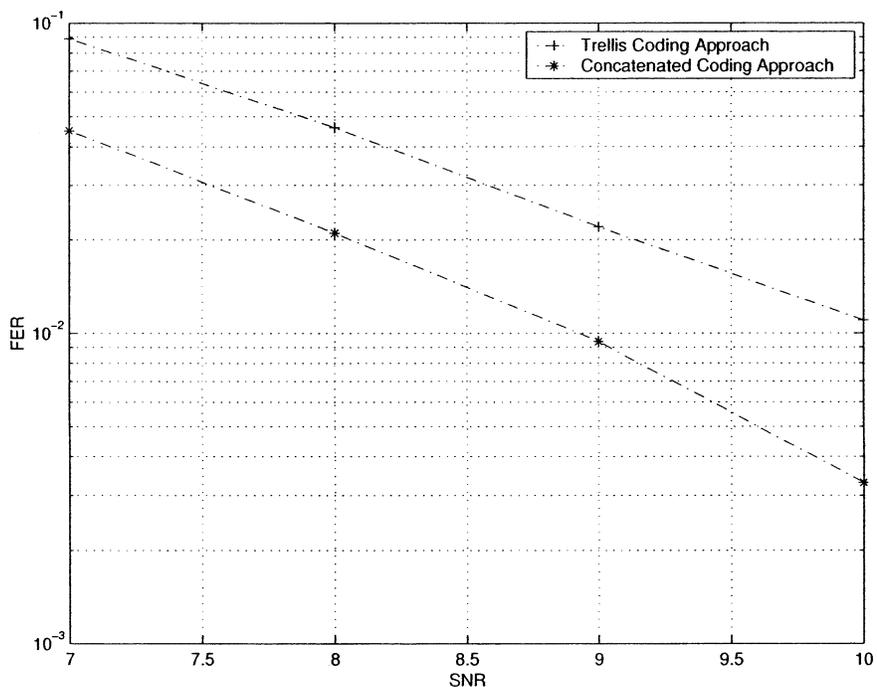
Fig. 10. Performance comparison of the serially concatenated coding approach and the trellis coding approach (BPSK).
