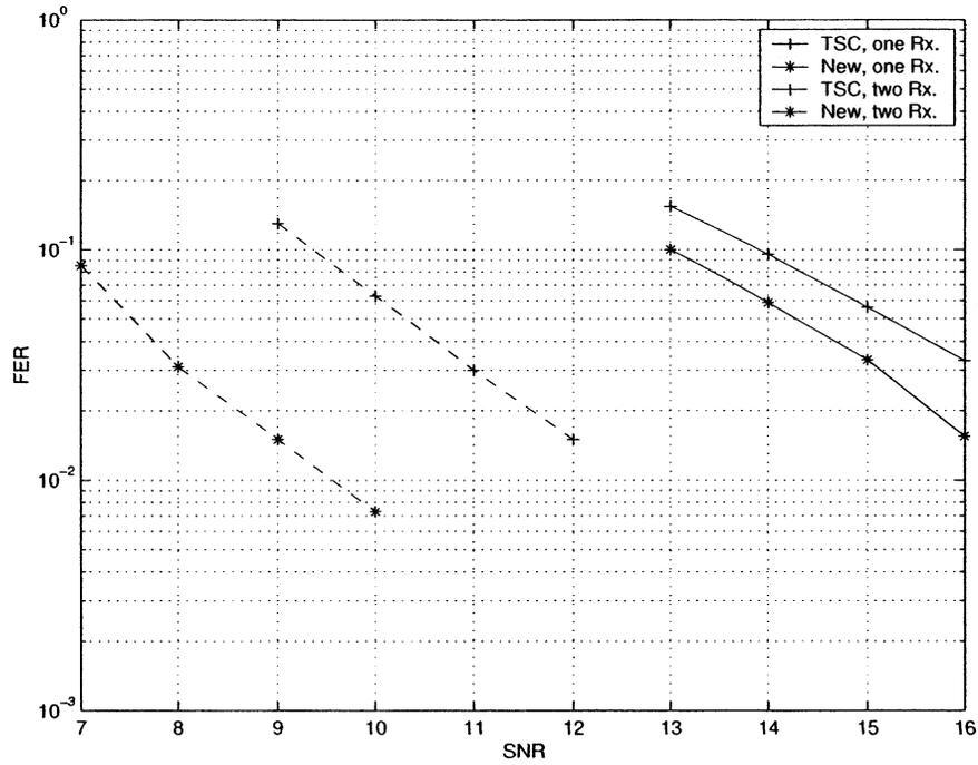
Fig. 11. Performance of two four-state QPSK STCs for  $L_t = 2$  and  $L_{\text{ISI}}=2$ .
