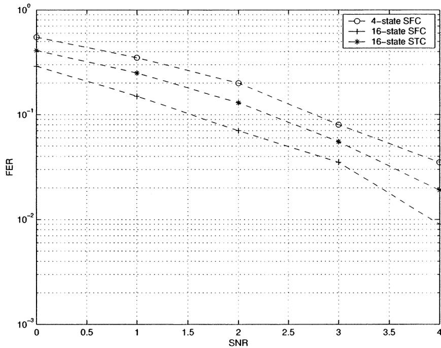
Fig. 7. Performance of BPSK STC and SFC with  $L_t = 2$ ,  $L_r = 2$ , and  $L_{ISI} = 3$ .
