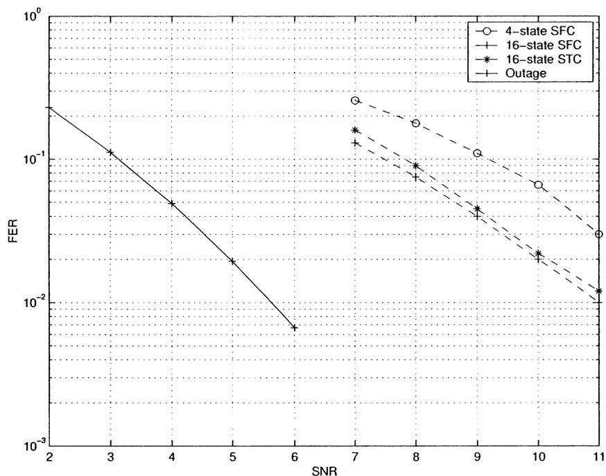
Fig. 6. Performance of BPSK STC and SFC with  $L_t = 2$ ,  $L_r = 1$ , and  $L_{ISI} = 3$ .
