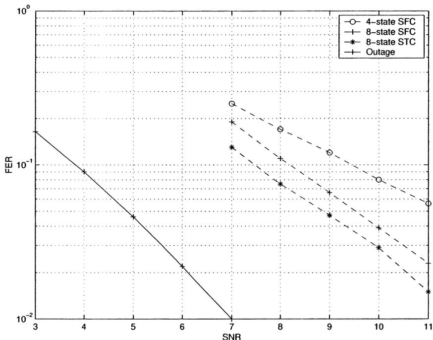
Fig. 5. Performance of BPSK STC and SFC with  $L_t = 2$ ,  $L_r = 1$ , and  $L_{ISI} = 2$ .
