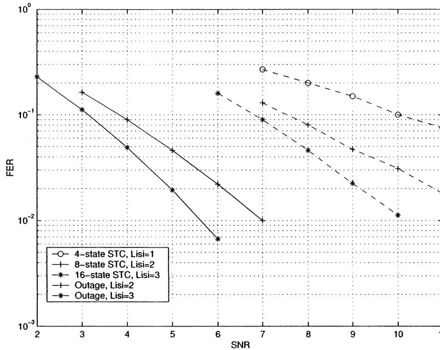
Fig. 3. Performance of four-state BPSK STC with  $L_t = 2$ , and  $L_r = 1$ .
