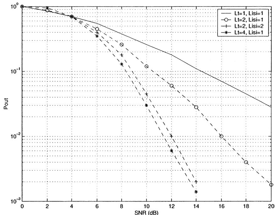
Fig. 1. The outage probability for systems with different number of transmit antennas, and different number of taps at transmission rate 2 bits/symbol.
