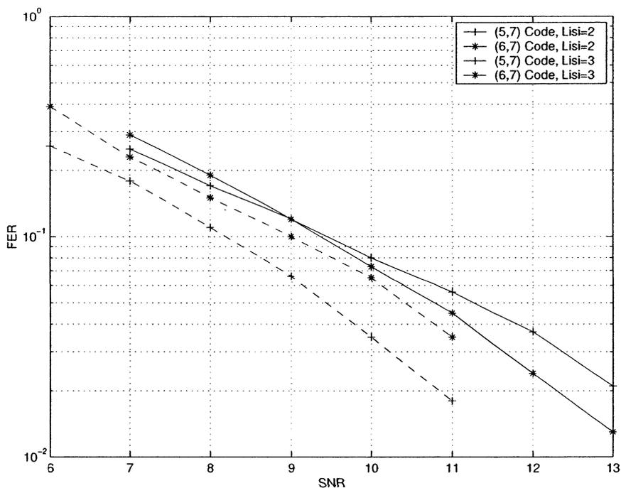
Fig. 9. Performance comparison of two four-state BPSK SFCs for  $L_t = 2, L_r = 1$ .
