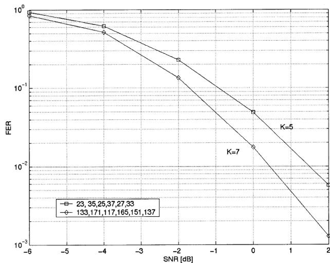
Fig. 6. Performance of algebraic QPSK space-time overlays with different constraint lengths ( $L_t = 3$ ,  $L_r = 3$ ).
