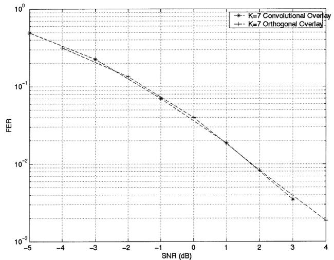
Fig. 3. Performance of the  $K = 7$  algebraic BPSK space-time overlay and the concatenated coding approach with inner orthogonal code and outer  $K = 7$  convolutional code with optimal free distance ( $L_t = 2, L_r = 2$ ).
