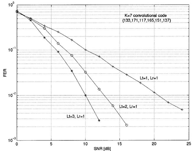
Fig. 4. Performance of  $K = 7$  algebraic QPSK space-time overlays with different number of transmit antennas ( $L_r = 1$ ).
