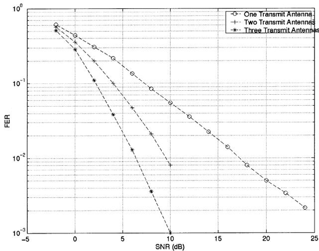
Fig. 1. Performance of  $K = 7$  algebraic BPSK space-time overlays with different number of transmit antennas ( $L_r = 1$ ).
