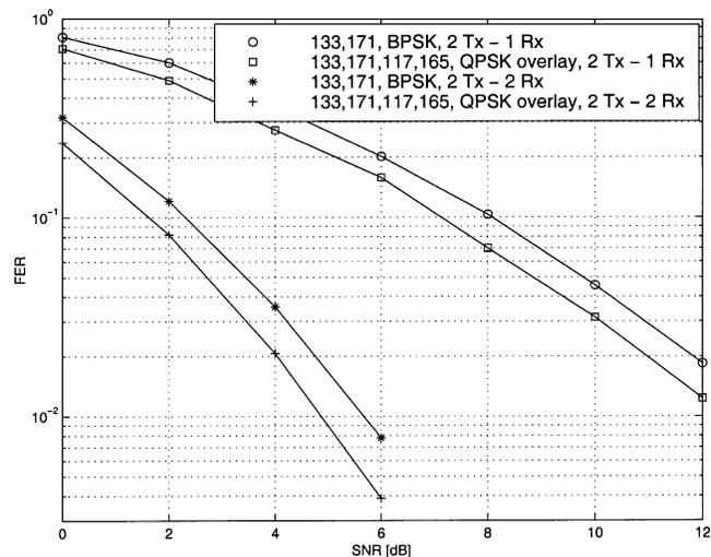
Fig. 7. FER performance comparison for the  $K = 7$  BPSK space-time convolutional code and the  $K = 7$  QPSK space-time overlay for  $L_t = 2$  transmit antennas and  $L_r = 1$  or  $L_r = 2$  receive antennas.
