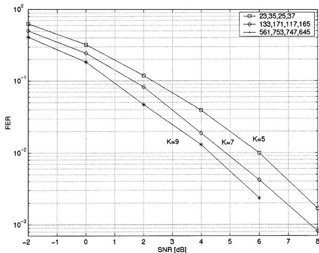
Fig. 5. Performance of algebraic QPSK space-time overlays with different constraint lengths ( $L_t = 2$ ,  $L_r = 2$ ).
