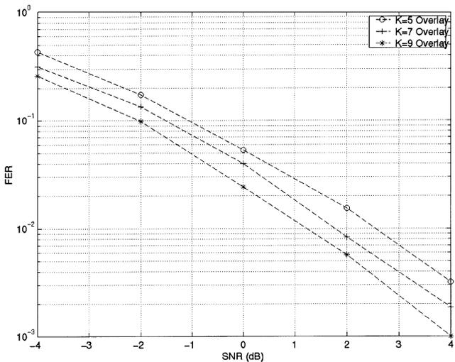
Fig. 2. Performance of algebraic BPSK space-time overlays with different constraint lengths ( $L_t = 2, L_r = 2$ ).
