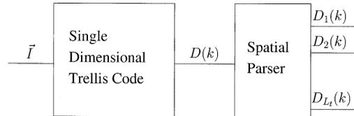
Fig. 3. Canonical construction for space-time coding.
