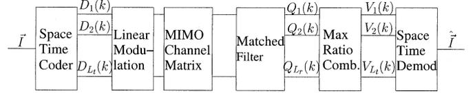
Fig. 1. Generalized MRC combiner implementation of the ML decoder.
