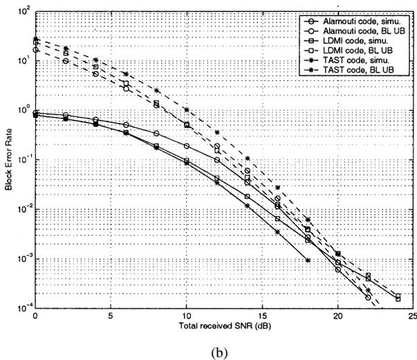
Fig. 2. Comparison of block error performance of  $R = 4$  bits PCU linear space-time block codes. (a) Union bound in (11). (b) BL union bound.
