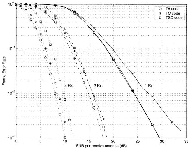
Fig. 5. Performance of space-time code designed for a more universal application, eight states,  $R = 3$  bits PCU,  $L_t = 2$ .
