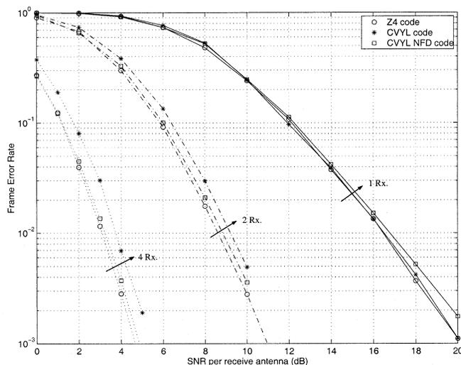
Fig. 4. Performance of space-time code designed for a more universal application, 32 states,  $R = 2$  bits PCU,  $L_t = 3$ .
