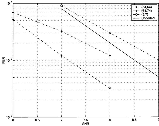
Fig. 3. Performance with phase randomization of BPSK ST codes with different  $\lambda_{\min}$  in line-of-sight channels with  $L_t = 2$  and  $L_r = 1$ .
