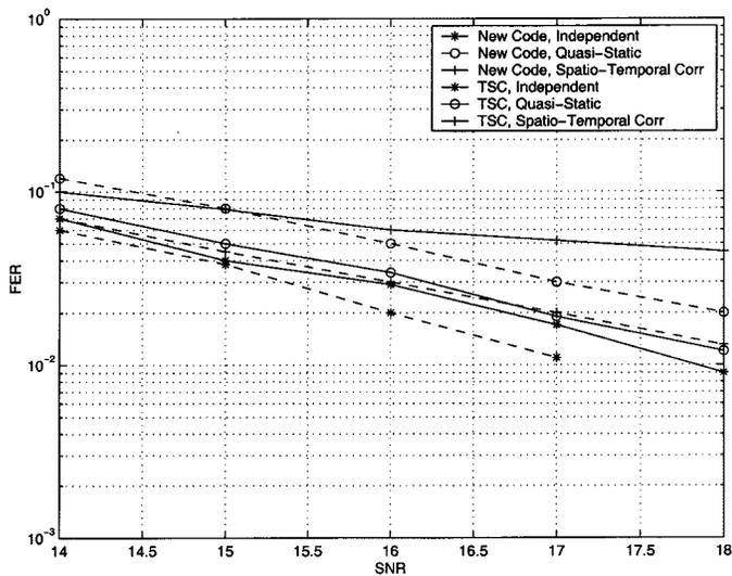
Fig. 8. Performance comparison of the new 16-state QPSK ST code and the TSC ST code with  $L_t = 2$ ,  $M = 2$ , and  $L_r = 1$  (the solid lines correspond to the TSC code and the dashed lines correspond to the new code).
