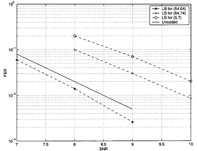
Fig. 2. Lower bound on the worst-case performance of BPSK ST codes with different  $\lambda_{\min}$  in line-of-sight channels with  $L_t = 2$  and  $L_r = 1$ .
