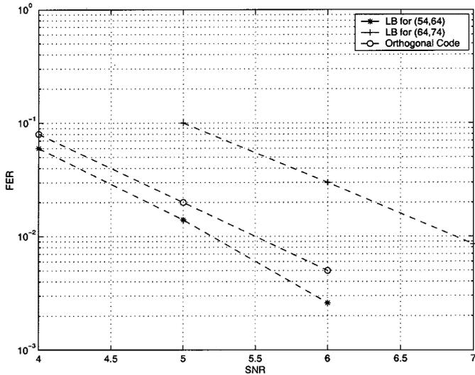
Fig. 4. Lower bound on the worst-case performance of BPSK ST codes with different  $\lambda_{\min}$  and  $G_2$  in line-of-sight channels with  $L_t = 2$ , and  $L_r = 2$ .
