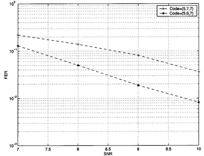
Fig. 6. Performance of four-state BPSK ST codes with phase randomization in line-of-sight channels with  $L_t = 3$  and  $L_r = 1$ .
