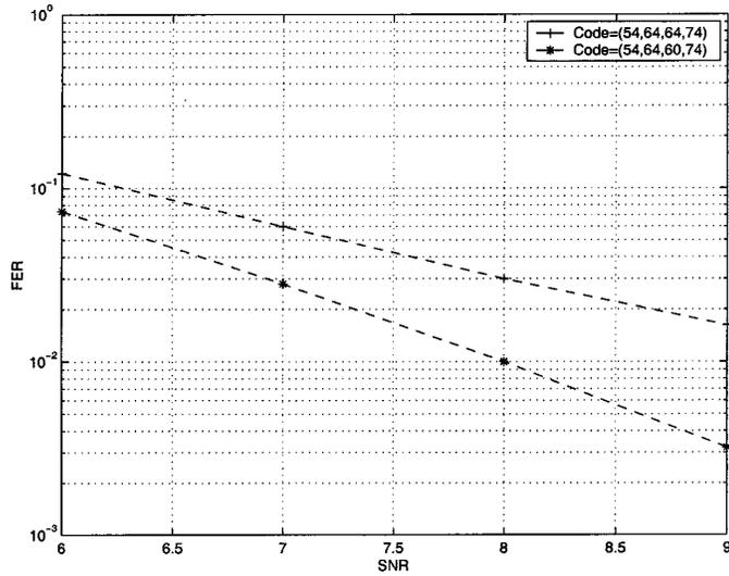
Fig. 7. Performance of eight-state BPSK ST codes with phase randomization in line-of-sight channels with  $L_t = 4$  and  $L_r = 1$ .
