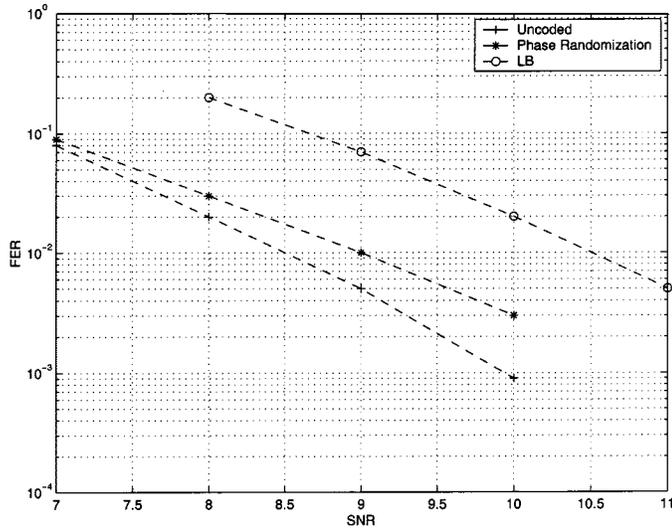
Fig. 1. Performance of the four-state (5, 7) BPSK ST code in line-of-sight channels with  $L_t = 2$  and  $L_r = 1$ .
