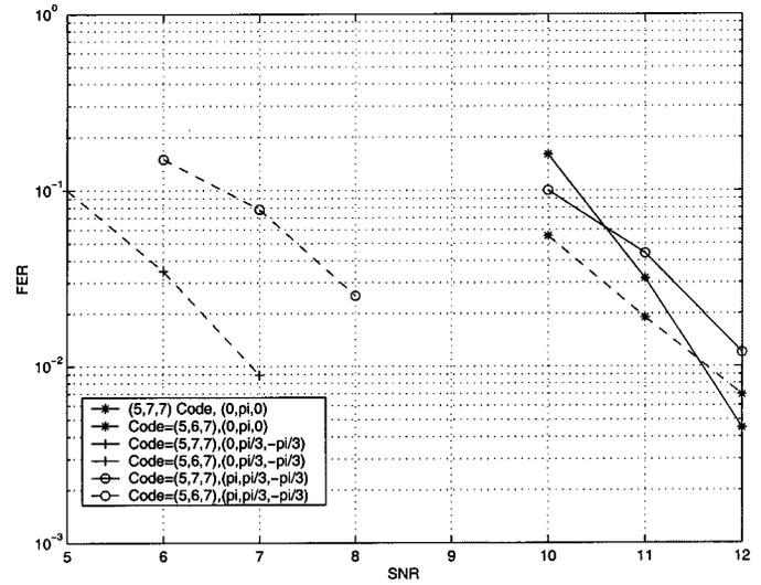
Fig. 5. Performance of four-state BPSK ST codes in line-of-sight channels with  $L_t = 3$ , and  $L_r = 1$  [the dashed lines correspond to the (5, 6, 7) code and the solid lines correspond to the (5, 7, 7) code].
