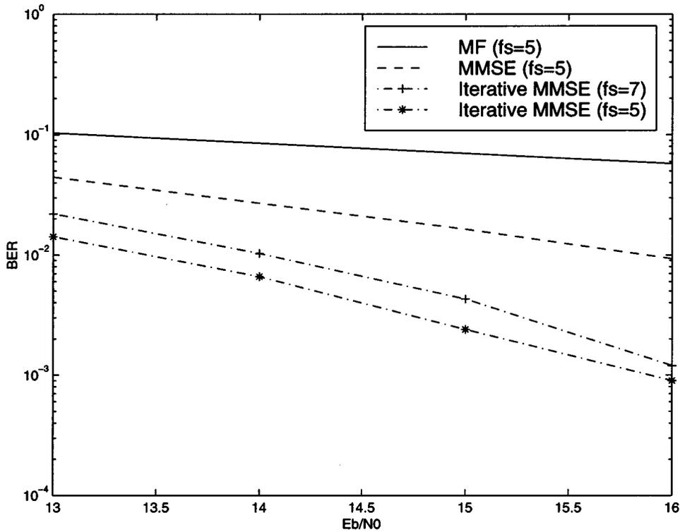
Fig. 7. Performance of the proposed multiuser receiver in Rayleigh fading channels.
