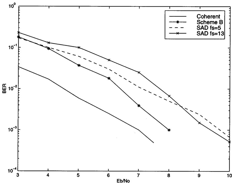
Fig. 6. Performance of the different channel estimation schemes for  $B_f T_s = 0.02$ .
