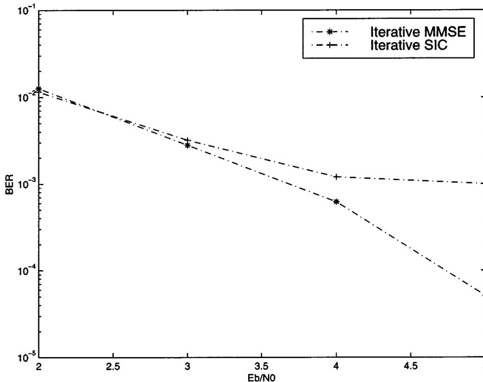
Fig. 4. Performance in the case of unequal power levels in AWGN channels.
