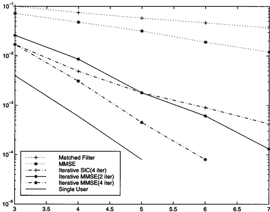
Fig. 2. Performance of the different CDMA receivers in AWGN channels.
