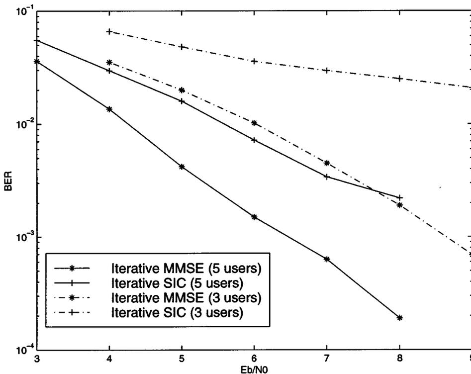
Fig. 3. Joint decoding of a subset of users in AWGN channels.
