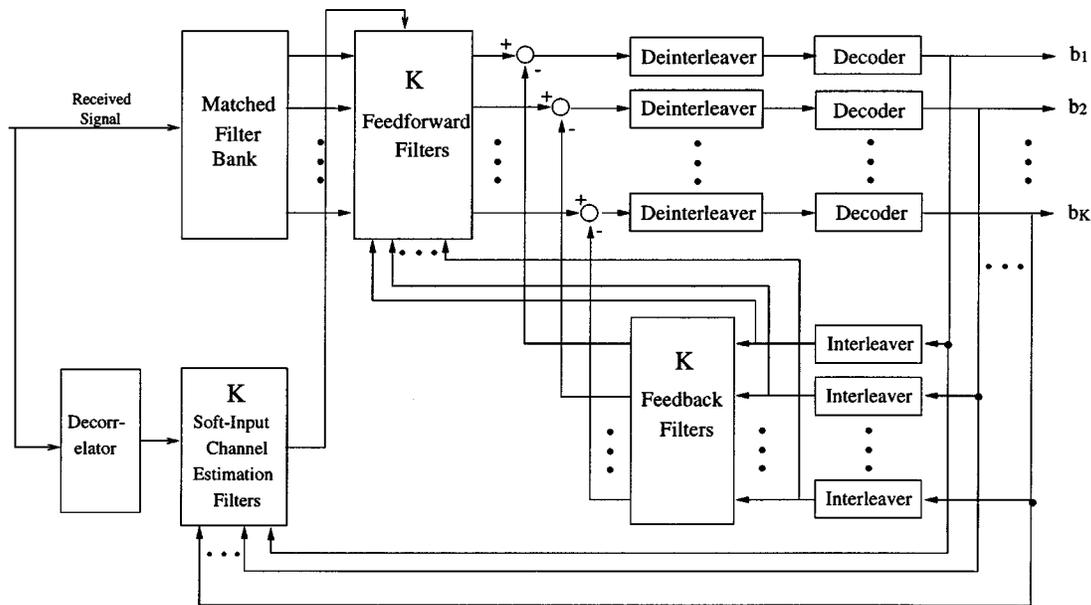
Fig. 1. Block diagram of the proposed multiuser receiver in fading channels.
