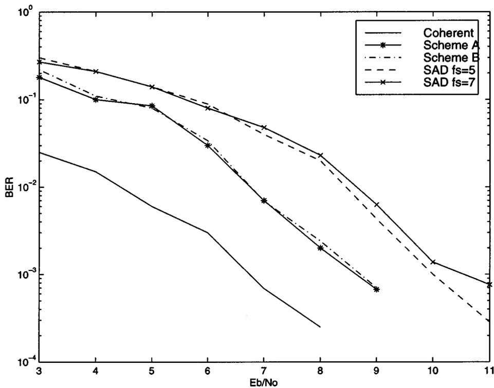
Fig. 5. Performance of the different channel estimation schemes for  $B_f T_s = 0.05$ .
