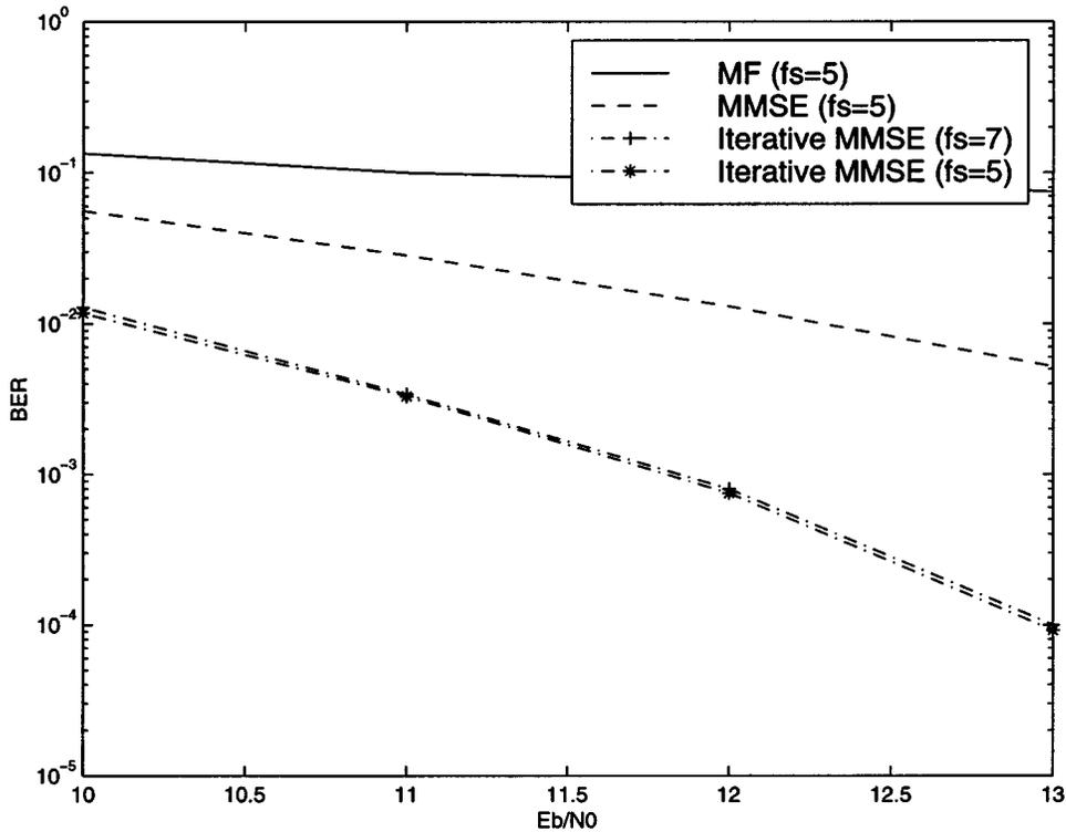
Fig. 8. Performance of the proposed multiuser receiver in Rician fading channels.
