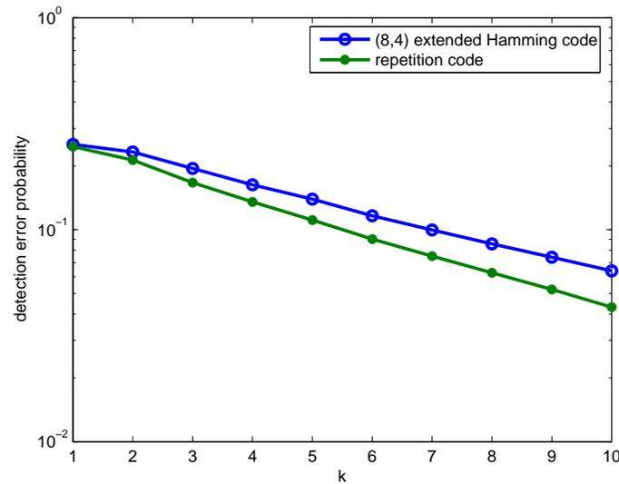
Fig. 6. Performance comparison between the  $(8, 4)$  extended Hamming code and the repetition code. The Bernoulli measurement noise has  $p = 0.2$  and the total transmit power  $P_{tot} = 0dB$ .
