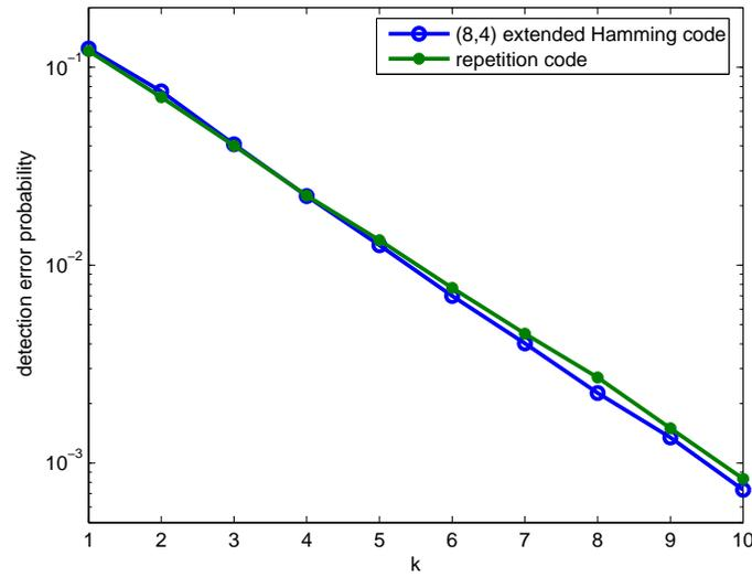
Fig. 5. Performance comparison between the  $(8, 4)$  extended Hamming code and the repetition code. The Bernoulli measurement noise has  $p = 0.05$  and the total transmit power  $P_{tot} = 0dB$ .
