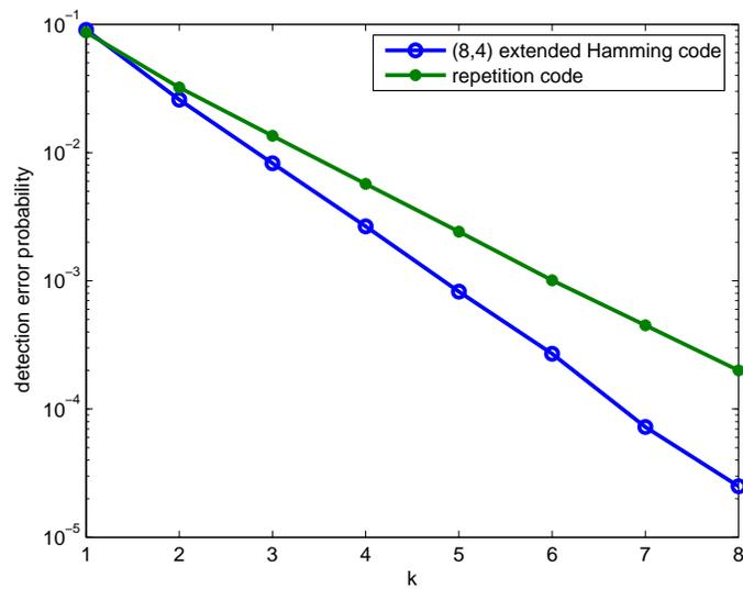
Fig. 4. Performance comparison between the  $(8, 4)$  extended Hamming code and the repetition code. The Bernoulli measurement noise has  $p = 0.01$  and the total transmit power  $P_{tot} = 0dB$ .
