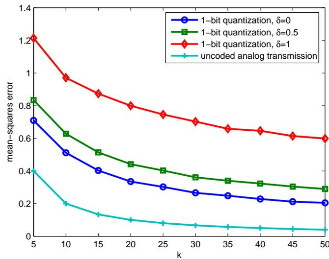
Fig. 2. Estimation performance of one-bit quantizers. Static MAC and  $P_{tot} = 10dB$ .
