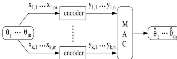
Fig. 1. A schematic illustrating decentralized inference over multiple access channels.
