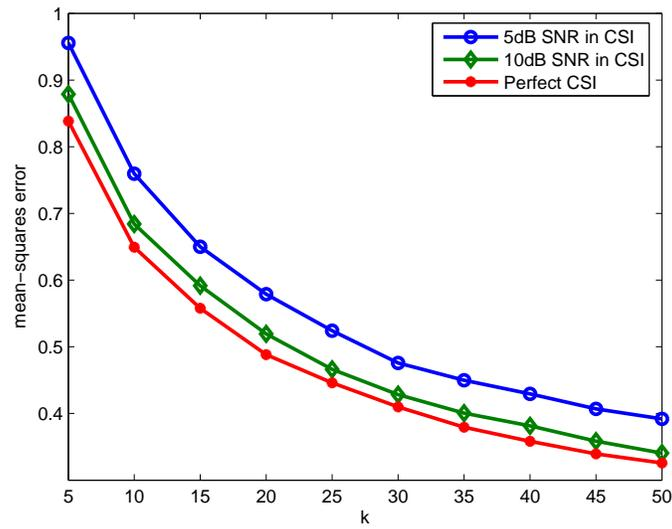
Fig. 3. Performance of one-bit quantizer ( $\delta = 0$ ) under noisy CSI feedback. Gaussian fading MAC and  $P_{tot} = 10dB$ .
