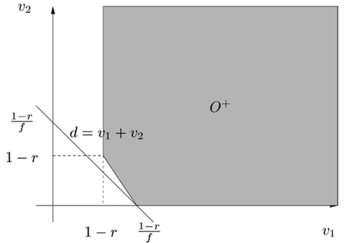
Fig. 12. Outage region for the DDF protocol with a single relay ( $f > 0.5$ ).
