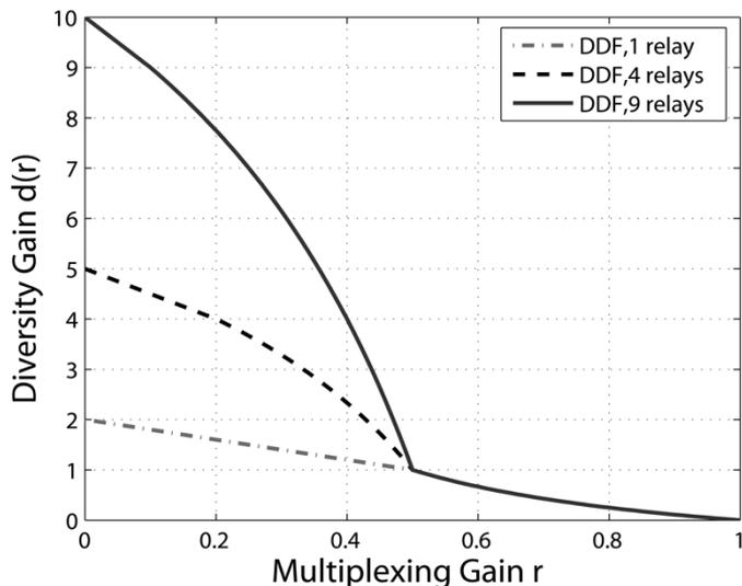
Fig. 5. Diversity–multiplexing tradeoff for the DDF protocol with different number of relays.
