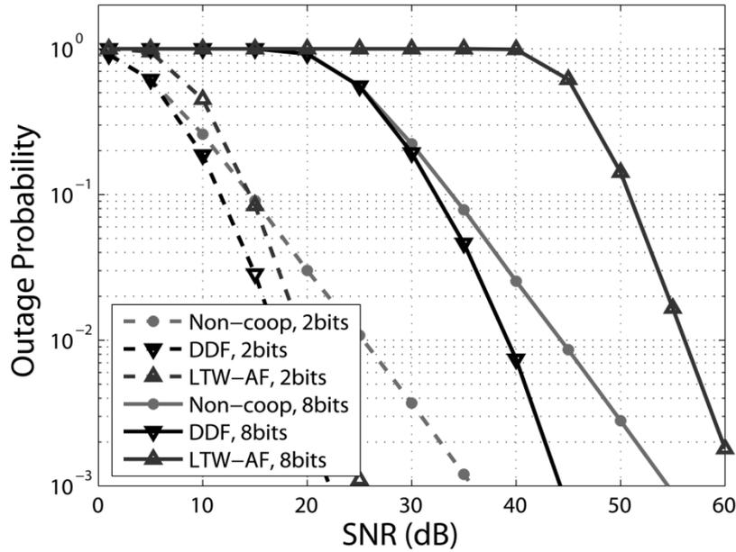
Fig. 8. Comparison of the outage probability for the DDF relay, LTW-AF, and noncooperative  $1 \times 1$  protocols ( $N = 2$ ).
