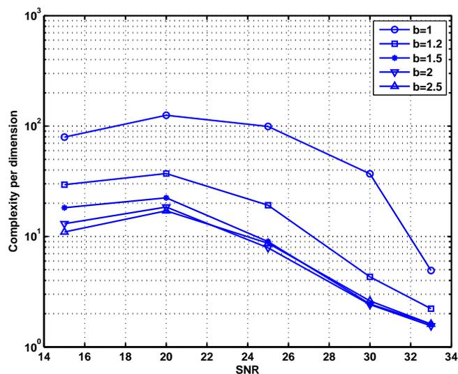
Figure 10: Performance-complexity tradeoff of MMSE-DFE Fano decoder in CMA-NAF setup (4 BPCU).
