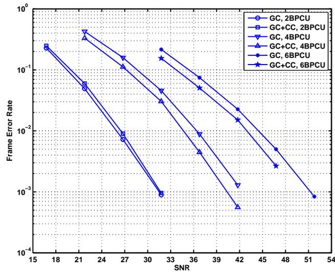
Figure 3: FER of NAF relay with Golden constellation, with and without CC outer code (denoted by GC+CC and GC).
