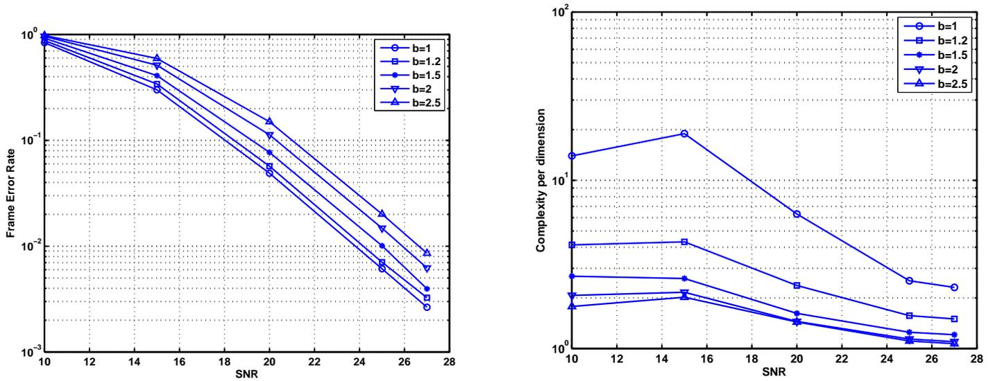
Figure 9: Performance-complexity tradeoff of MMSE-DFE Fano decoder in the CMA-NAF setup (2 BPCU).
