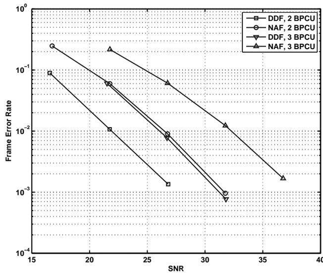
Figure 5: FER of DDF relay protocol (with 3 segments) versus NAF relay protocol.
