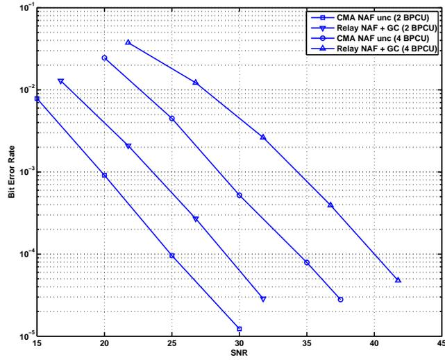
Figure 8: BER of CMA-NAF protocol with uncoded QAM versus Relay NAF protocol with Golden constellation.
