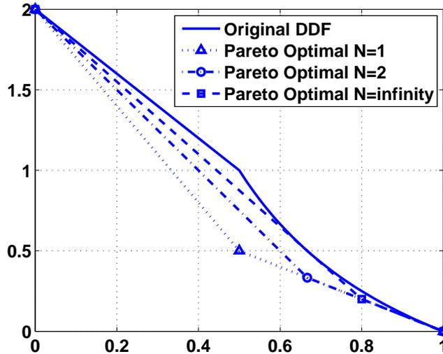
Figure 1: DMT of Pareto optimal DDF protocol with  $N = 1, 2$  and  $\infty$ .
