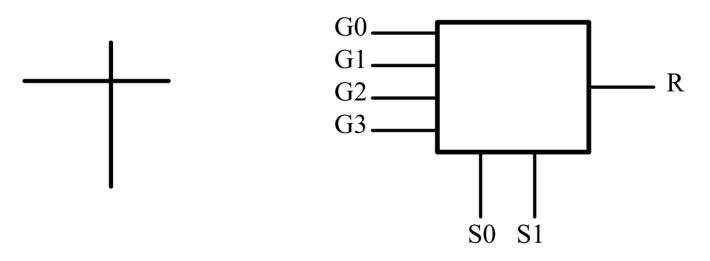
This Unit Can perform any of the logic functions of 2 inputs
