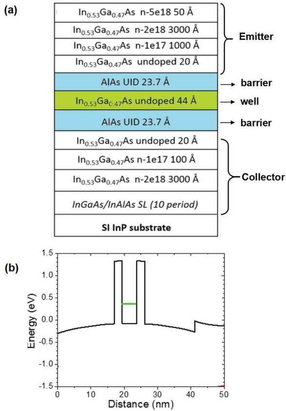
Fig. 1. (a) Epitaxial layer structure for the RTD. (b) Band structure showing the first quasi-bound level [8].
