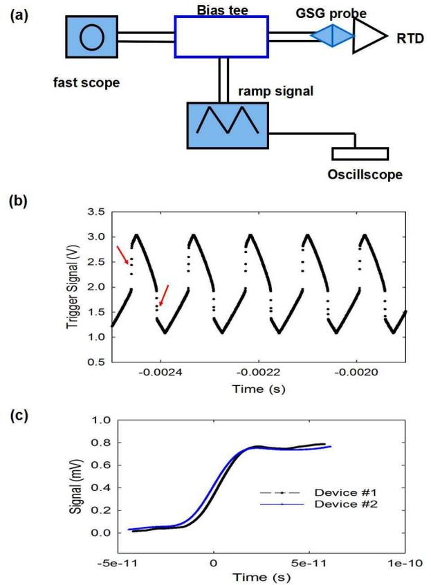
Fig. 2. (a) Switching-time measurement setup. (b) Ramp signal monitored with the slow-speed oscilloscope. Red arrows mark the peak-to-valley (the left arrow) and valley-to-peak (the right arrow) switching events, respectively. (c) Peak-to-valley switching waveform measured with the fast-speed scope.
