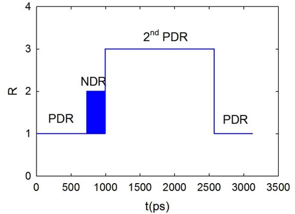
Fig. 5. Operational stages of the RTD device during a cycle of ramp signal determined by calculating the bias voltage of RTD,  $V_D$ . If device operates in PDR region, then  $R$  is set as 1; if in NDR region,  $R$  is set as 2; and if in the second-PDR region,  $R$  set as 3. Note the shaded area of the NDR region indicates the oscillation of  $V_D$  between the PDR and NDR regions.
