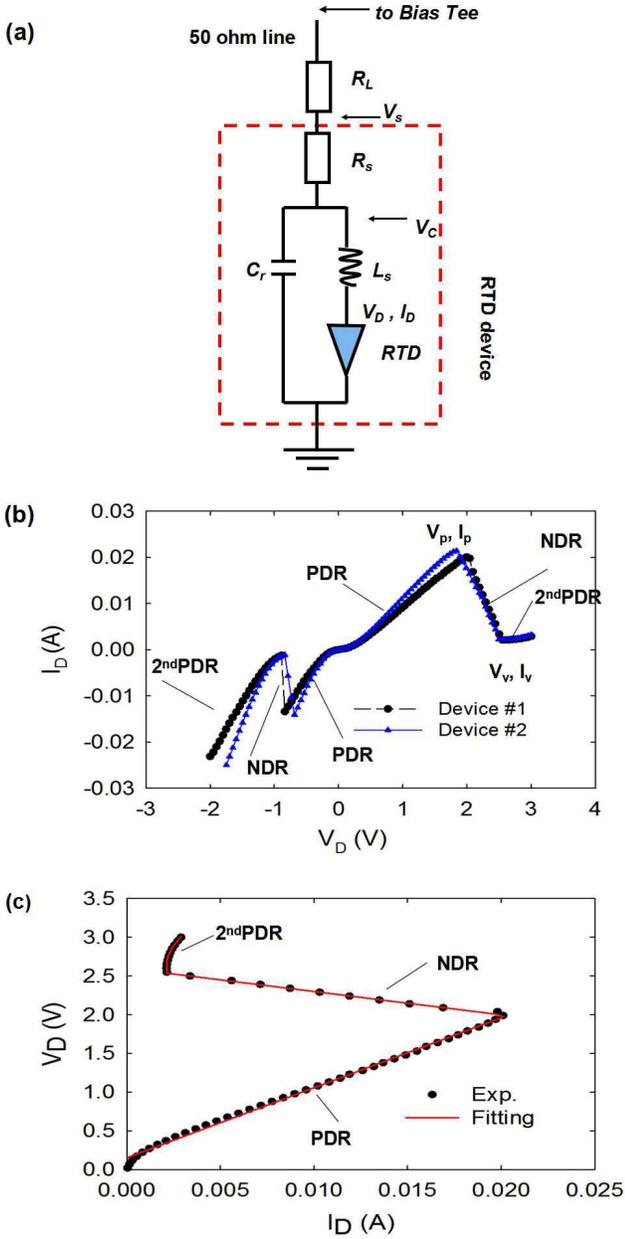
Fig. 3. (a) Large-signal model for RTD. (b) Experimental  $I$ - $V$  curve of RTD (device 1). (c) Voltage-current curve (forward) and its piecewise fitting functions in PDR, NDR, and the second-PDR regions.
