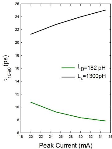
Fig. 6. Influence of peak current on switching time simulated with the large-signal model.
