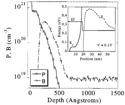
Fig. 1. SIMS profile of B and P dopants for the high current density Si  $p^+ - i - n^+$  Esaki diode prior to *ex situ* annealing. The inset displays the calculated band diagram where  $E_F$  is the quasi-Fermi level,  $E_C$  is the conduction band edge and  $E_V$  is the valence band edge.
