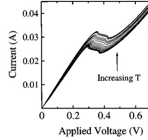
Fig. 4. Variable temperature  $I$ - $V$  curves of a  $40 \times 40 \mu\text{m}^2$  Si Esaki tunnel diode after a 60 s anneal at 775 °C. Measurement temperatures ranged from 4.2 to 325 °K. The variation of peak voltage versus peak current yields a series resistance of 8  $\Omega$ .
