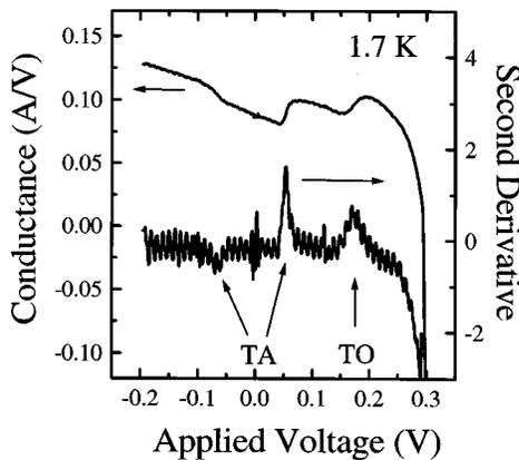
Fig. 6. Conductance,  $dI/dV$  (left axis) and the second derivative,  $d^2I/dV^2$  (right axis) of the LTMBE grown Si Esaki diode from Fig. 4 taken at 1.7 K. After correcting for series resistance, we attribute the inflections to contributions from the TA (18.4 meV) and TO (57.6 meV) phonons to the tunneling current.
