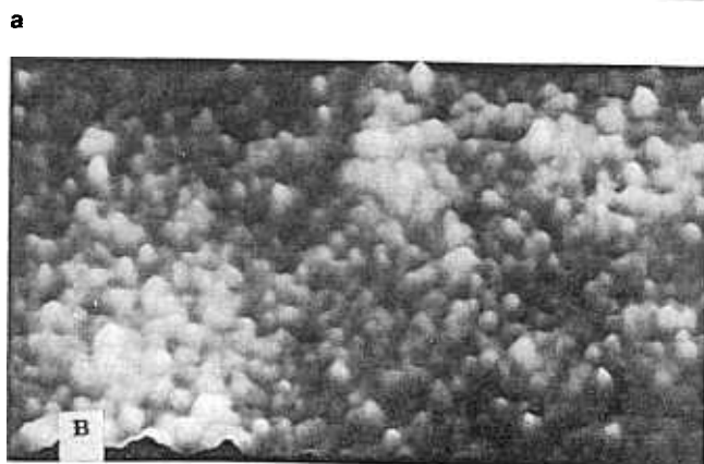
Fig. 2. (a) STM image of the surface of a GaAs (100) buffer layer. The tunneling voltage was 2.8 V, applied to the sample, and the tunneling current was 70 pA. The As terminated surface shows rows of missing As dimers along the [\bar{1}10] direction that are spaced 1.6 nm apart, corresponding to the 4X spacing. The corrugation is 0.2 nm, and (b) 90 nm \times 50 nm STM scan of the surface after four monolayers of \text{In}_{0.35}\text{Ga}_{0.65}\text{As} have been deposited. The crystal axes are the same as in (a). The tunneling voltage was 3.0 V, applied to the sample, and the tunneling current was 30 pA. The surface is covered with islands roughly 3.2 nm in diameter and with an average corrugation of 0.6 nm. Examination with RHEED shows this surface to have a diffuse (1 \times 1) pattern and a 0.7% relaxation of the surface lattice constant.
