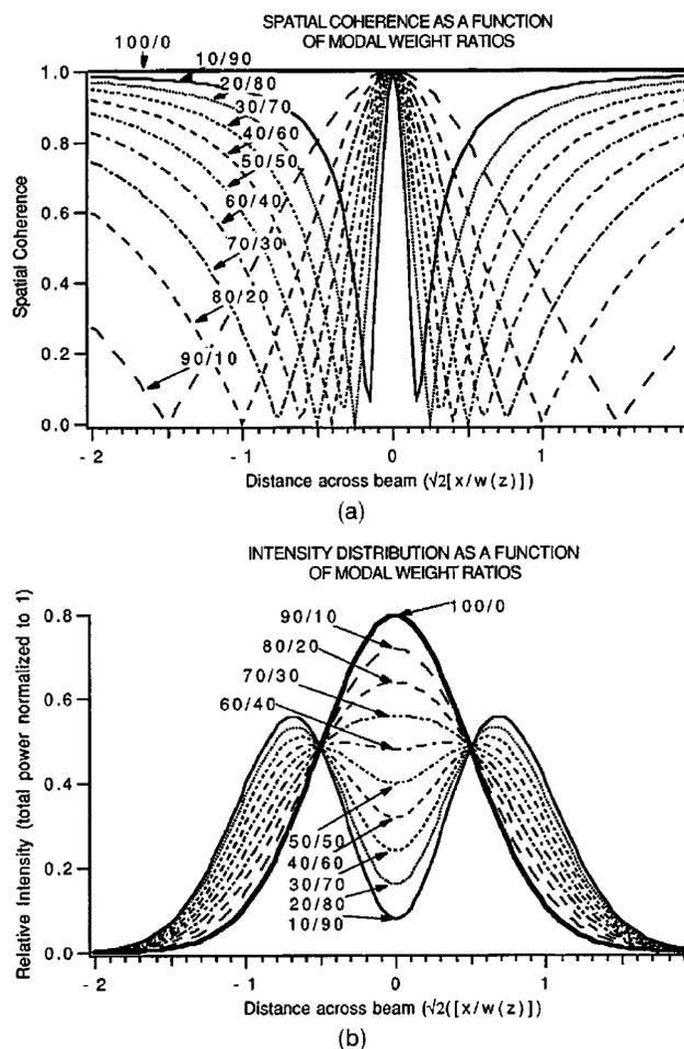
Fig. 3. (a) SCF's and (b) intensity distributions for various percentages of the total energy in fundamental/first modes.
