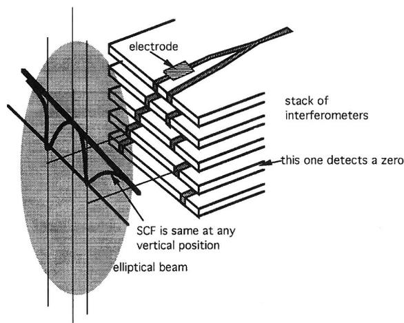
Fig. 11. Stack of interferometers. Data in this case are intended for the receiver that is second from the bottom. Others can detect but are programmed to ignore the data.
