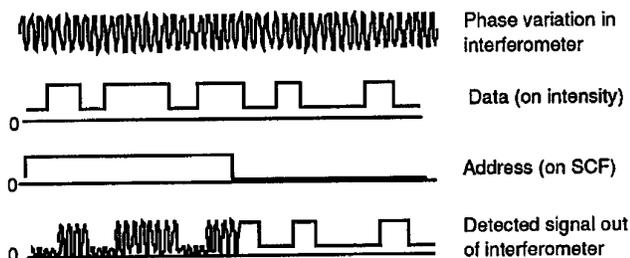
Fig. 10. Example of signals in a multiplexed system, in which data are carried by intensity modulation and the address is carried on the same beam on the spatial-coherence modulation.
