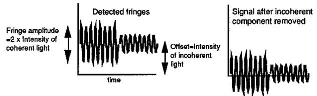
Fig. 8. Intensity is modulated, but spatial coherence is detected. Ambient (incoherent) light adds a uniform dc offset to the fringes.
