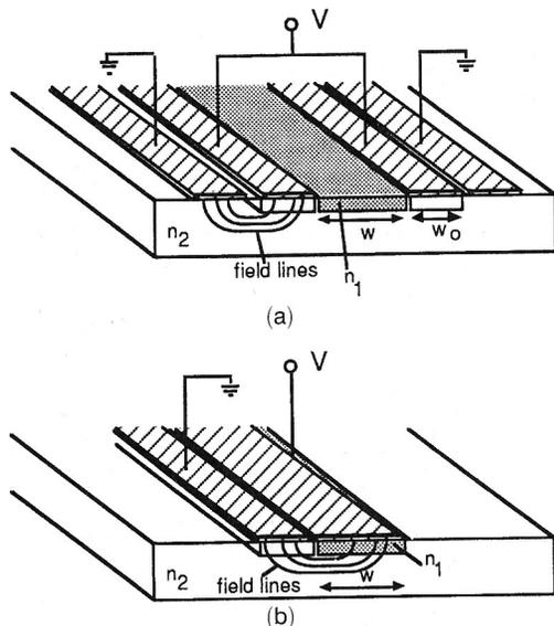
Fig. 5. Two proposed external modulator structures: (a) center passive core, with electro-optically controlled outrigger waveguides; (b) single core, where waveguide  $\Delta$  is electro-optically controlled.
