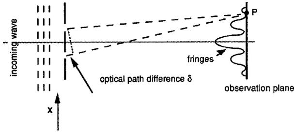
Fig. 1. Young's double-slit geometry for measuring spatial coherence.
