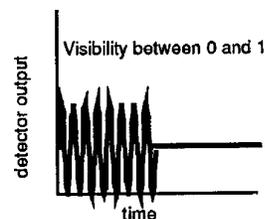
Fig. 9. Spatial coherence (but not intensity) is modulated; spatial coherence is detected. Energy found at the fringe frequency gives a one or a zero.
