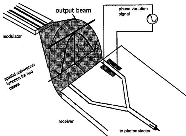
Fig. 7. The receiver distinguishes between zero coherence (two modes present) and perfect coherence (one mode present).
