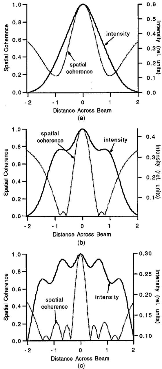
Fig. 4. Examples of arbitrary cases in which more than just the first two modes are present: (a) The first three modes are present in the energy ratio of 70:20:20 (zeroth:first:second); (b) the relative strengths of the first three modes are 40:30:30; (c) the first five modes present in equal weights.
