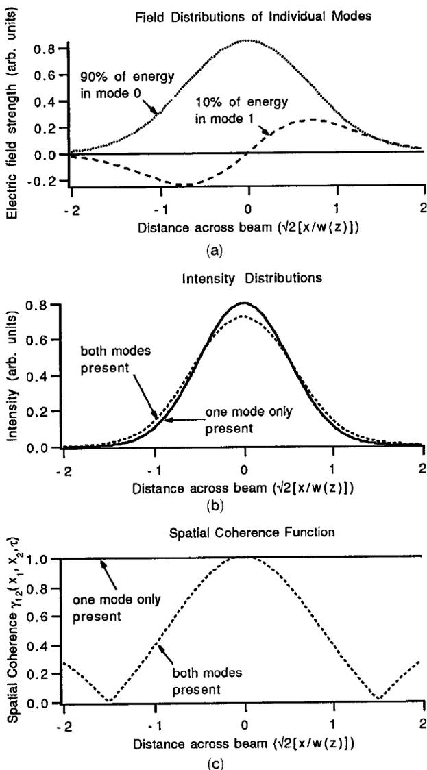
Fig. 2. (a) Field distributions for first two modes as a function of distance across the beam. Ninety percent of the total energy is carried in the fundamental mode. (b) Two intensity distributions, one with all energy carried in the zeroth mode, the other with a 90:10 energy distribution as in the first graph. (c) SCF's for the same two cases.
