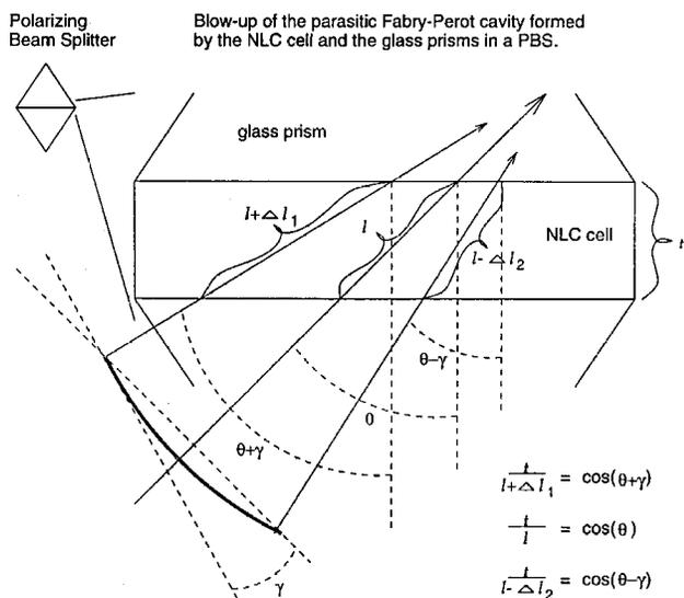
Fig. 9. Distance traveled by light at the edges of a curved wave front through a Fabry-Perot cavity differs from that at the center of the beam. Assuming a spherical wave front,  $\Delta l_1$  and  $\Delta l_2$  give the changes in the electrical distance for a given  $\gamma$ .
