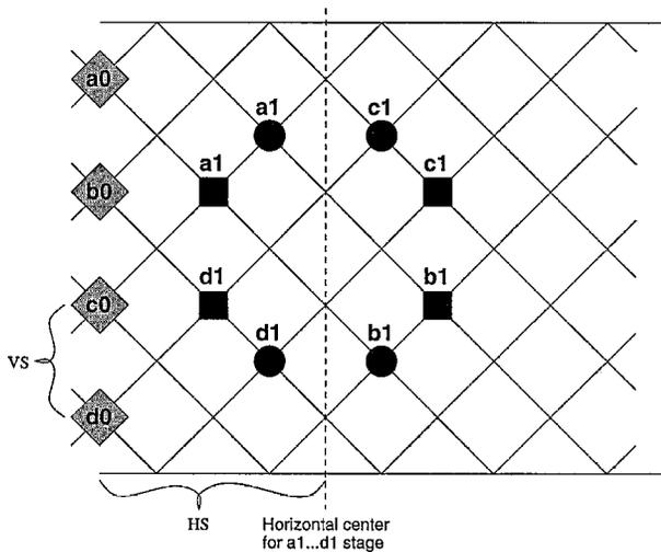
Fig. 10. Two possible placements for a perfect-shuffle connection with  $[a_0 + c_0 \rightarrow a_1, a_0 + c_0 \rightarrow b_1, b_0 + d_0 \rightarrow c_1, b_0 + d_0 \rightarrow d_1]$ . The next stage can occupy the intersections covered by either the squares or the circles. The horizontal centers of both possible placements occur at the same place. VS and HS for either of these placements are also shown.
