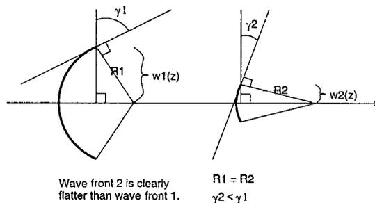
Fig. 8. Radius of curvature of the wave front is not an adequate measure of its flatness. Instead, the angle  $\gamma$  between the normal to the direction of propagation of the beam and the tangent to the wave fronts at the edge of the beam is used.
