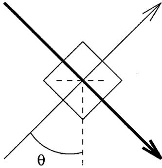
Fig. 3. Inputs and outputs for the  $2 \times 2$  switches are not parallel unless extra optics are incorporated. For the acousto-optic switch,  $\theta = 45^\circ$ . For the ferroelectric liquid-crystal switch,  $\theta \approx 68^\circ$ .
