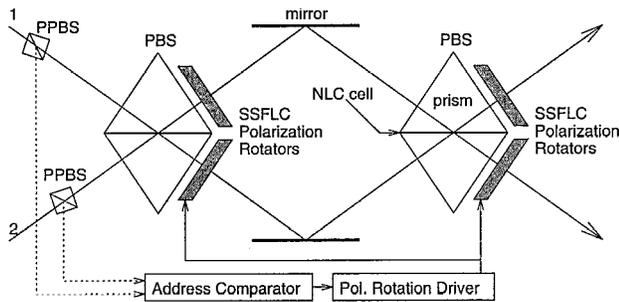
Fig. 5. Configuration of the ferroelectric liquid-crystal  $2 \times 2$  switch.
