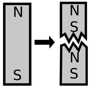
Figure 4: Magnetic Dipoles
