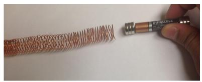
Figure 1: Finished Solenoid Track and Battery Train
