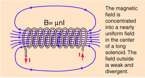
Figure 2: Solenoid and its Magnetic Field (Source: <u>http://hyperphysics.phy-astr.gsu.edu/hbase/magnetic/solenoid.html</u>)
