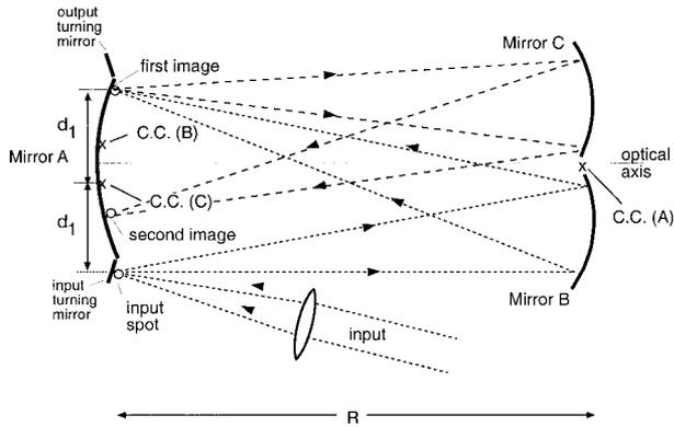
Fig. 1. Original White cell consists of three spherical mirrors, of identical radii of curvature  $R$ , separated by  $R$ . The centers of curvature (C.C.) for each mirror are shown. A spot introduced into the White cell via the input turning mirror produces a series of spots on mirror A.
