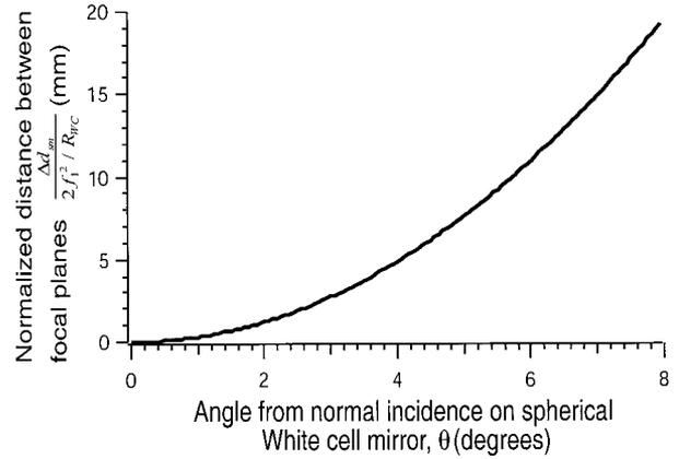
Fig. 6. Normalized astigmatism versus angle of incidence  $\theta$  in the binary cell according to expression (14). The astigmatic image distance is normalized to  $R_{WC}/2f_1^2$ .
