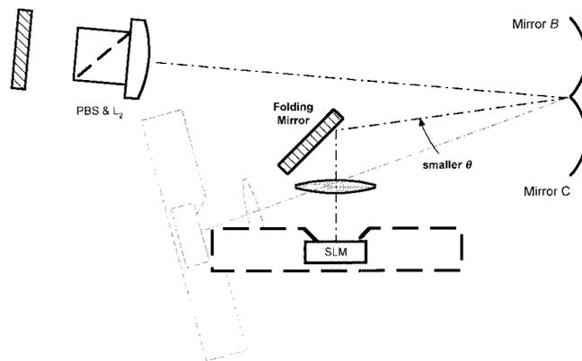
Fig. 8. Top view of the binary cell with a flat mirror to fold the path of the SLM branch. Folding the light path will allow us to reduce the angle of incidence  $\theta$  on the White cell mirrors B and C.
