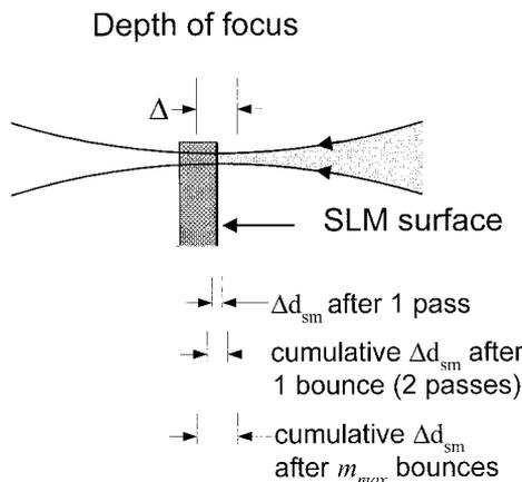
Fig. 7. Depth of focus due to beam divergence at the SLM surface. The depth of focus depends on the size of the beam waist as well as the wavelength of light. The astigmatic image distance  $\Delta d_{sm}$  after one, three, and  $m_{max}$  passes is also shown.
