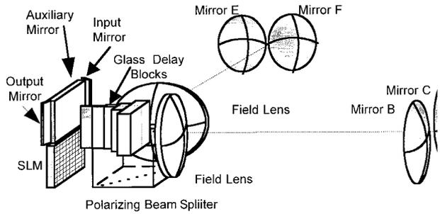
Fig. 3. Three-dimensional view of the TTD White cell with a binary architecture that uses glass blocks.
