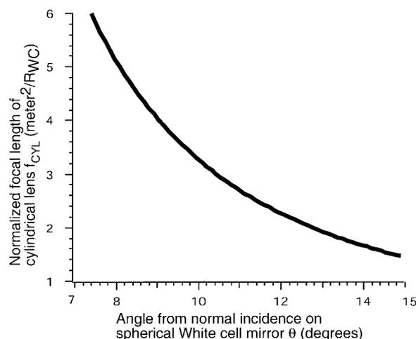
Fig. 11. Normalized focal length of the cylindrical lens needed to correct for the astigmatism as a function of the angle of incidence on the White cell (spherical) mirrors,  $\theta$ . The focal length in this plot is normalized by dividing by the radius of curvature  $R_{WC}$  of the White cell mirrors.
