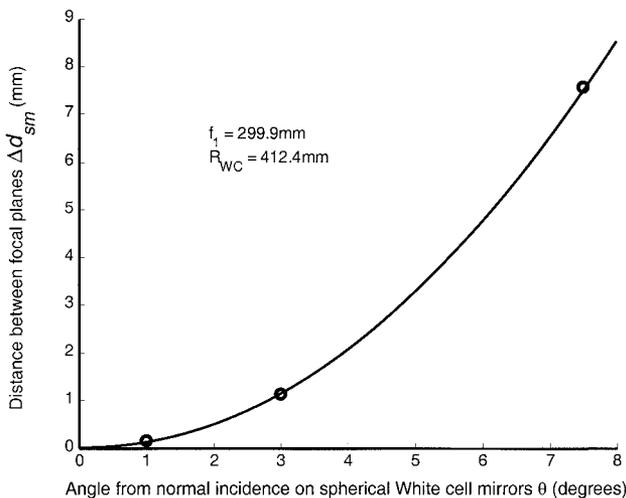
Fig. 13. Astigmatism versus angle of incidence  $\theta$  in the binary bell of the design of Table 1. The circled data points on the graph denote  $\Delta d_{\text{sm}}$  for the angles  $7.5^\circ$ ,  $3^\circ$ , and  $1^\circ$ .
