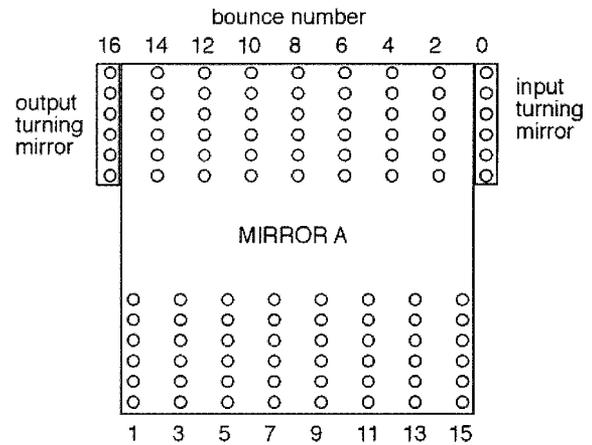
Fig. 2. Spot pattern produced on mirror A by six input beams undergoing 16 bounces apiece.
