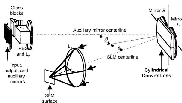
Fig. 10. Three-dimensional view of a binary White cell with a cylindrical mirror to compensate for non-Seidel astigmatism.
