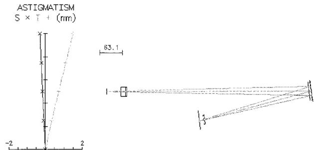
Fig. 15. Cylindrical lens is placed in front of the spherical mirror to correct the astigmatism. The focal length is  $f_{CYL} = 24$  m for  $\theta = 7.5^\circ$ . The astigmatism for an object on axis is now 0.00144 mm.
