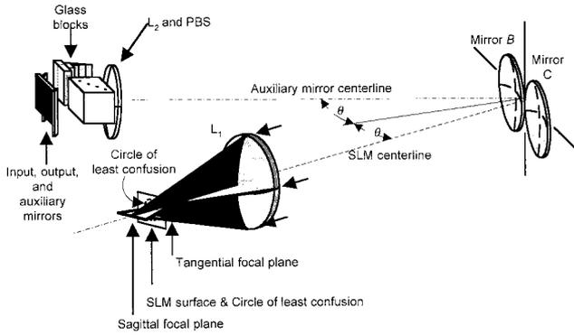
Fig. 5. Astigmatic focus at the plane of the SLM surface. The astigmatic image creates tangential and sagittal focal planes. The surface of the SLM is located in between these two focal planes at the circle of least confusion for best imaging.
