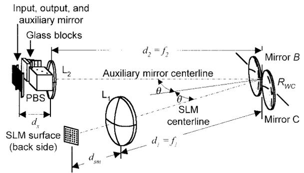
Fig. 4. Three-dimensional view of the new binary cell configuration. PBS, polarizing beam splitter.
