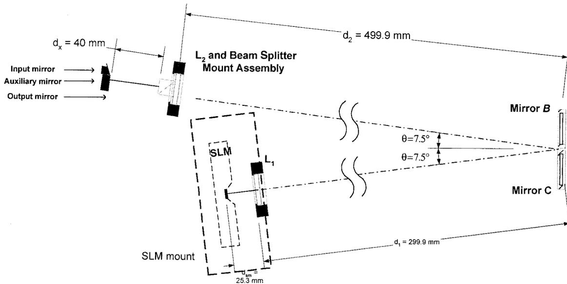
Fig. 12. Design configuration of binary cell TTD controller of the design of Table 1. Note that the SLM surface is embedded deep within the SLM housing (heavy dashed line), making it physically impossible to place the turning mirrors in the same plane as the SLM surface.
