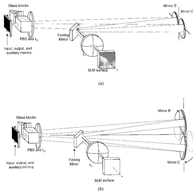
Fig. 9. Three-dimensional view of a binary White cell (a) with a folding mirror and (b) vertically oriented mirrors B and C.
