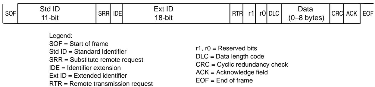
**Figure 1. Data Frame (With Extended Identifier)**
