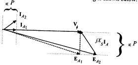
Since the power supplied by the motor is constant, the quantity  $I_{\mathcal{A}}\cos\theta$ , which is directly proportional to power, must be constant. Therefore,
