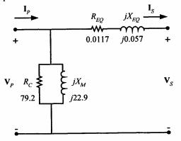
(b) If this transformer is operating at rated load and 0.90 PF lagging, then current flow will be at an angle of  $-\cos^{-1}(0.9)$ , or  $-25.8^{\circ}$ . The voltage at the primary side of the transformer will be
