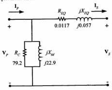
(b) If this transformer is operating at rated load and 0.90 PF lagging, then current flow will be at an angle of  $-\cos^{-1}(0.9)$ , or  $-25.8^{\circ}$ . The voltage at the primary side of the transformer will be
