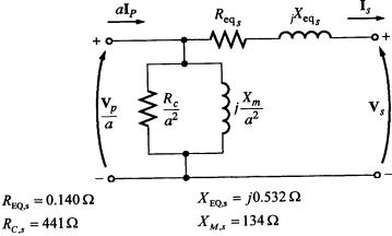
(b) To find the required voltage regulation, we will use the equivalent circuit of the transformer referred to the secondary side. The rated secondary current is
