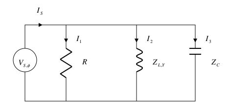
$$V_{S,\phi} = \frac{220}{\sqrt{3}} = 127.02 \angle 0^{\circ} V$$
