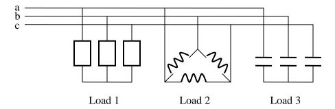
Load 1 are three lamps, each rated 100 watts at 120 volts. Load 2 are three inductors, each having an inductance of 0.1 Henry. Load 3 are three capacitors, each having a capacitance of 100  $\mu$ F.
