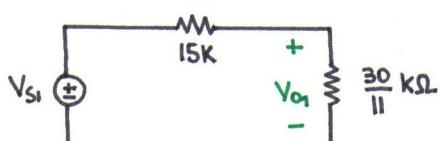
$$V_{o1} = \frac{R_{EQ} \cdot V_{S1}}{(5k\Omega + 10k\Omega) + R_{EQ}} = \frac{30/11}{15 + 30/11} \cdot 10 = \frac{20}{13} = 1.538V$$
