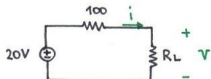
$$\left\{ \begin{array}{l} V = \frac{R_L}{R_L + 100} \cdot 20V \\ \text{for } 500\Omega \leq R_L \leq 3000\Omega \end{array} \right.$$
