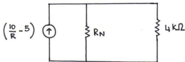
Since  $R_T = R_N$  and max power delivered  $\leftrightarrow R_T = 4\text{k}\Omega$
