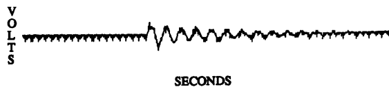
Fig. 24: Measured Bridge rectifier output following rated load drop with modified second harmonic filter.
