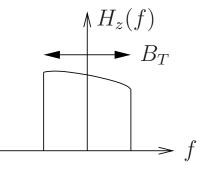
Applying the baseband filter to a baseband signal is equivalent to applying the passband filter to a passband signal:
