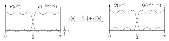
The resulting Q(z) is non-negative and satisfies the amplitude-symmetry condition  $Q(e^{j\omega}) + Q(e^{j(\pi-\omega)}) = 1+2\epsilon$ . We will make up for the additional " $2\epsilon$ " gain later. The procedure by which  $H_0(z)$  can be calculated from the raised halfband Q(z), known as "spectral factorization," is described next.
