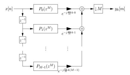
Because it is a linear operator, the downsampler can be moved through the adders and the (time-invariant) scalings  $e^{-j\frac{2\pi}{M}k\ell}$ . Finally, the Noble identity is employed to exchange the filtering and downsampling. The  $k^{th}$  filterbank branch becomes:
