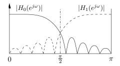
The QMF design rules imply that all filters in the bank are directly related to the "prototype" filter  $H_0(z)$ , and thus we might suspect a polyphase implementation. In fact, one exists. Using the standard polyphase decomposition of  $H_0(z)$ , we have
