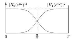
• Design of Orthogonal PR-FIR Filterbanks via Halfband Spectral Factorization: Recall that analysis-filter design for orthogonal PR-FIR filterbanks reduces to the design of a real-coefficient causal FIR prototype filter  $H_0(z)$  which satisfies the power-symmetry condition
