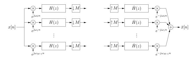
In an *M*-branch critically-sampled uniformly-modulated filterbank, the  $k^{th}$  analysis branch extracts the sub-band signal with center frequency  $\omega_k = \frac{2\pi}{M}k$  via modulation and lowpass
