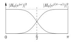
Power complementarity follows from the second orthogonal PR design rule, which implies  $|H_1(e^{j\omega})| = |H_0(e^{j(\pi-\omega)})|$ . Plugging this into the previous equation, we find
