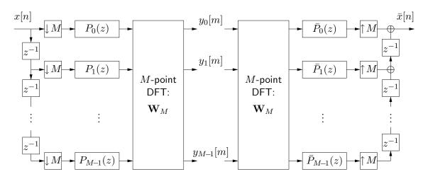
Recall that the standard implementation performs modulation, filtering, and downsampling, in that order. The polyphase/DFT implementation reverses the order of these operations; it performs downsampling, then filtering, then modulation (if we interpret the DFT as a two-dimensional bank of "modulators"). We derive the polyphase/DFT implementation below, starting with the standard implementation and exchanging the order of modulation, filtering, and downsampling.
