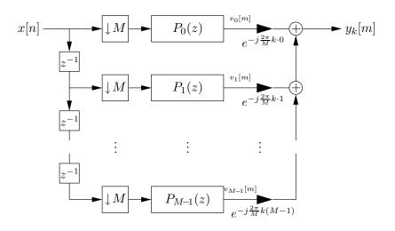
Observe that the polyphase outputs  $\{v_{\ell}[m], \ell = 0...M-1\}$  are identical for each filterbank branch, while the scalings  $\{e^{-j\frac{2\pi}{M}k\ell}, \ell = 0...M-1\}$  are different for each filterbank branch since they depend on the filterbank branch index k. Thus, we only need to calculate the polyphase outputs  $\{v_{\ell}[m], \ell = 0...M-1\}$  once. Using these outputs we can compute the branch outputs via
