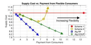
Fig. 4. Algorithms RP and COUP perform better with increasing flexible consumer penetration in the system. In RP,  $\epsilon_n(t) \sim \mathcal{U}\left(-\epsilon,\epsilon\right)$ , where  $\epsilon$  is set to be 1% of the average of the optimal common price. In COUP,  $\gamma$  is set to be 10% of the average of the common price.
