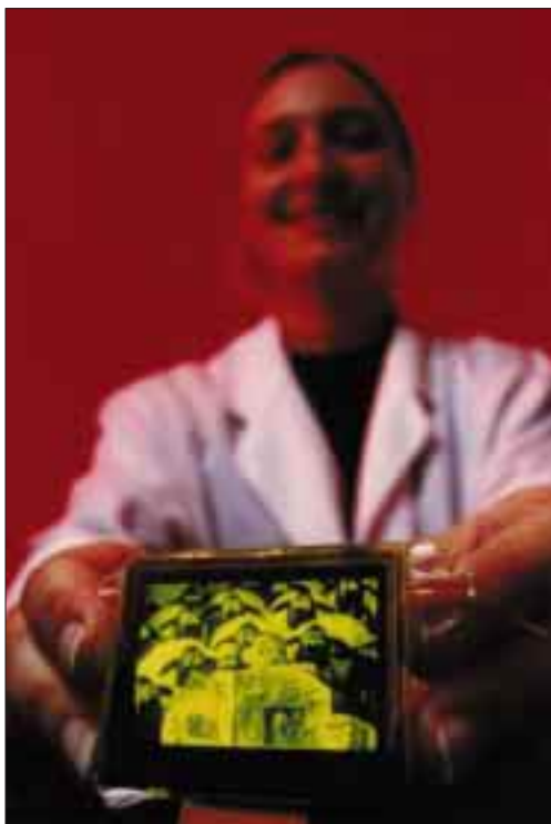
Plastic fantastic – a polymer LED display in which the pixels have poly(phenylene vinylene) as the active element
